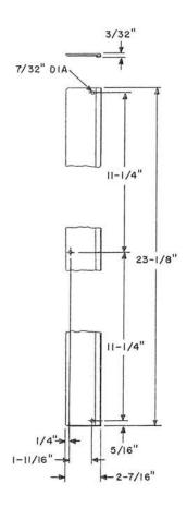
A light olive gray enamel finished sheet metal flat section arranged for closing the ends of one or a group of 1A1 Cable Terminal Sections.
