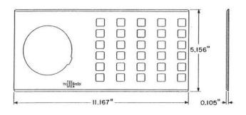
Clear plastic face plates, each containing openings to accommodate a dial and key buttons on associated telephone set.
