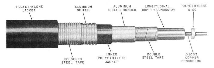
This cable is the same as CA-3185 except as follows: The cable has a PASP sheath with an additional moisture barrier under the inner jacket consisting of longitudinal aluminum tape with bonded overlap. The cable weighs approximately 0.35 pound per foot and is approximately 0.84 inch in diameter.
