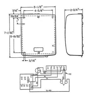
Common battery set having a metal base on which are mounted a C4A Ringer, a 425B Network, a 426A Electron Tube, and a terminal block. Has a light olive gray plastic cover assembled to the base.
