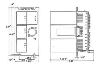
Terminal panel has 40 terminals, arranged in 4 rows of 10 each, numbered 1 to 40.
