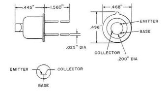
An N-P-N germanium alloy junction transistor assembled in a hermetically sealed metal can.
