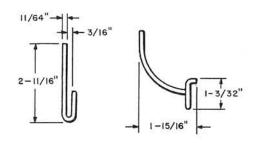
Metal support used in GA, GB, and GC type cable terminal boxes. Mounting screw and washer are furnished. Comcode: 100 666 627
