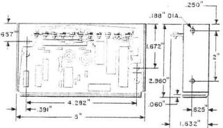
A three-stage transistorized amplifier consisting of resistors, transistors, and capacitors assembled on a printed wiring board within a metal frame. A terminal plate of insulating material containing 11 screw type terminals is assembled to the wiring board.
