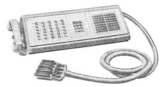
16AW1: A desk surface type telephone console having 6 control buttons (Night Service, Position Release, Transfer, Release Destination, Hold and Start), 24 pickup buttons, and a DSS field for 80 stations. Overall dimensions are approximately 24.090 inches wide by 9.000 inches deep by 4.250 inches high. Designed for use with the 800A PBX. Provides Series 200 and 300 service.
