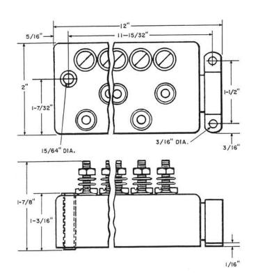
Molded terminal block containing twenty 2A1A Protector Units and binding posts. Screws and lockwashers are provided for mounting.
