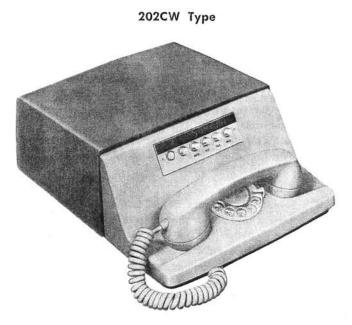
Data Set 202CW5: An FM transmitting-receiving data terminal integrated with a telephone set in a single housing and provides normal point-to-point voice transmission and reception of serial digital information. Optional two- or four-wire operation is provided. The set operates at a speed of 1200 to 1800 bits per second. Each is equipped with a D6AA-61 Cord. When set is used on four-wire operation, a D34B-61 Cord is required and must be ordered separately.
