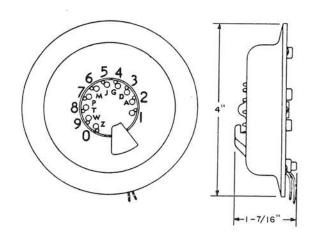
Provided with an insulated black case and an insulated finger wheel. The finger wheel when rotated causes a pair of contacts to make and break thus permitting impulses to be sent into the dial system offices. Two black terminal leads approximately 9 inches long connected to the contact spring are furnished.
