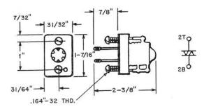
Oxidized copper disc type varistor with an enveloping lacquer finish. Consists of four 3/4-inch diameter discs clamped to a base of insulating material provided with terminals.
