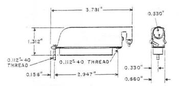
153A: Consists of a KS-16689L6 Plug and a terminal block having eight terminals arranged for screw connections. Comcode: 100 000 629
