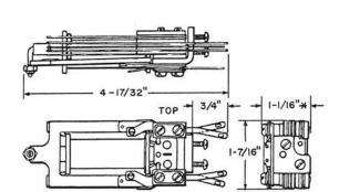
\*This dimension varies according to the number of contact springs and winding terminals on the indi-vidual relays.
