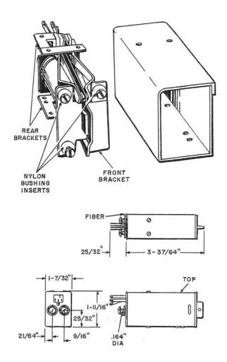
B-type relays differ from E- and H-types in that they are provided with a micrometer screw adjustment feature which permits extremely accurate adjustments to be made. Individual covers are provided and each has a removable cap which may be placed in position without affecting the adjustment of the relay. Relays are supplied dust and crosstalk proof. When crosstalk shielding is not required, dust-proof covers are supplied.
