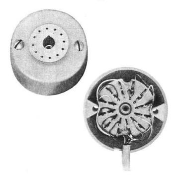
Nonflush-type jack consisting of a block of insulating material containing twelve spring contacts equipped with quick contact terminals. The associated 504A Plug can be inserted in one position only. Overall dimensions are 1.345 inches high by 2.540 inches in diameter. Two wood screws are provided for mounting.
