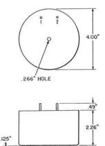
Consists of a winding on two moly-permalloy power cores encapsulated in epoxy. Arranged to mount by means of a 0.266 inch clearance hole through the center of the inductor. Mounting hardware is not furnished.
