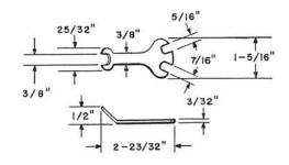
A triple wrench for use on nuts of binding posts of receivers and transmitters. Comcode: 100 750 462
