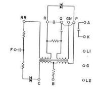
Consists of a transformer, capacitors, resistors, and varistors potted in a metal case. Terminal screws are shipped loose.
