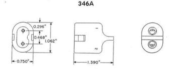
Polarized plug consisting of a black, molded body equipped with two pin type contacts which mate with the No. 471A jack. Each contact is designed to accommodate a No. 130 or similar cord tip, and set screws are provided for holding the cord tie and has two notches to provide partial locking with the springs of the jack.
