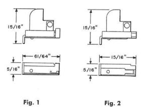
319C: Dummy plug of brown insulating material with a metal guide which is provided with a spring for locking
