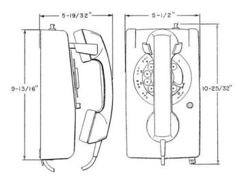
Transmission features and external appearance same as 554 and 556 type sets except for key located on front and top of housing. The key on the front of set is a combined turn and push button key for switching and signaling purposes. The exclusion type key, projecting through the top of the housing, provides the means for disconnecting an extension set by manually raising the plunger. When the hand set is replaced on the switch hook, the exclusion key is returned to its normal position.
