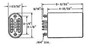
Consists of a shell type coil with silicon steel core potted in metal case. Closest recommended mounting centers are 1-3/4 inches by 3-3/16 inches. For electrical characteristics, see table at end of inductor descriptions.
