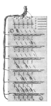
Consists of a molded plastic block equipped with horizontally and vertically aligned rows of terminal connectors, commonly referred to as clip terminals, arranged to receive pigtailed 446F Diodes. Diodes are not furnished and must be ordered separately. A 714B Tool is required for diode installation and must be ordered separately.
