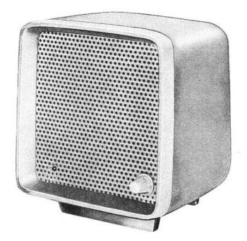
106A: Consists of a loud speaker and amplifier assembled on a chassis within a metal housing 5.500 inches wide by 4.625 inches deep by 6.1875 inches high having a green finish. The knob on the right controls an ON-OFF switch and a gain control potentiometer. A 2Y Lamp behind a red jewel indicates the ON condition.
