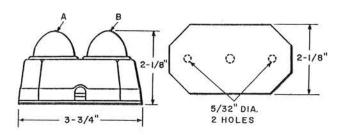
Two lamp indicator equipped with beehive lenses colored as indicated below. Housing is of insulating material and has a light olive gray finish.
