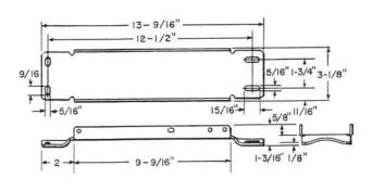
Metal bracket for mounting NC10 and NC16 and NF10
