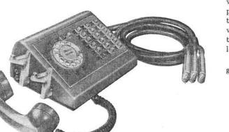
General purpose key sets providing either two- or fourwire service. They are equipped with a line switch which provides six transfer contacts, a relay for switching between two- or four-wire circuits, an 8C Dial, a 4010B Network, an N1A Ringer, a G3AR type hand set, a D120C type mounting cord, and the apparatus shown in the following table.
