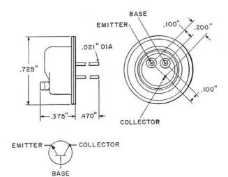
An N-P-N silicon nonepitaxial mesa transistor assembled in a hermetically sealed metal can.
