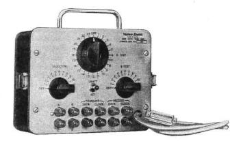
A portable test set used to make out-of-service installations and routine trouble checks on data sets. Operation of the switches simulates various business machine actions to the data set. A two-position toggle switch is used to control automatic answering circuits of the data sets equipped for unattended operation.
