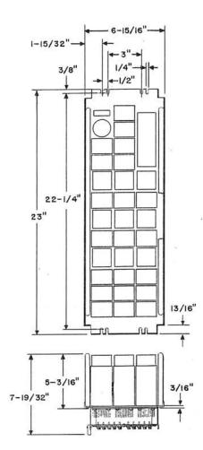
Terminal panel has 200 terminals, arranged in 5 groups of 40 terminals each. Each group is arranged in 4 rows of 10 each, numbered 1 to 40.
