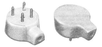
A four contact plug having a plastic shell. Equipped with a cord fastener which holds the cord in place while the spade tips are being connected and also anchors the mounting cord in the assembled plug. Used with portable telephone sets having 2, 3, and 4 conductor mounting cords.
