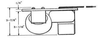
Consists of a harmonic generating transformer, a capacitor, an inductor, and a combined tuning, isolating, and load transformer mounted on a panel of insulating material. Flexible terminal leads are provided for input connections.
