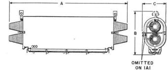
Each consists of a base of molded insulating material, reinforced with metal and equipped with cable sheath clamps and brackets for strand mounting. A cover of molded insulating material is assembled to the base by means of wire clips.
