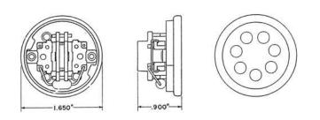
LA2: A bipolar, central armature, composite magnetic type, light weight receiver unit. Terminals in the rear of the frame are arranged for electrical connections by means of screw and spade tip, spring contact, or soldered leads.
