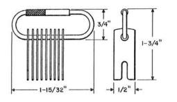
Consists of 67A through 67P Gauges assembled on a holding ring.
