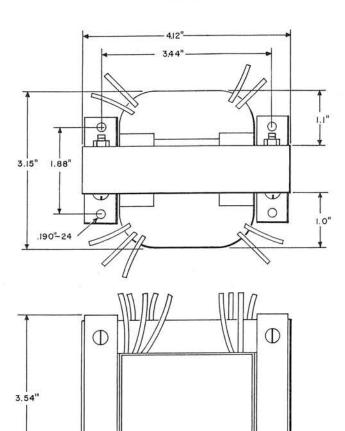
Shell type transformer having a silicon steel core clamped between metal brackets which provide a means for mounting.
