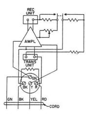
Consists of a T1 Transmitter Unit, a receiver unit, a polarity guard, and a H4CT spring-type cord. Provides receive amplification at noisy locations. Equipped with a press-to-listen switch which when depressed reduces transmitter output and increases the gain of the receiver amplifier. A potentiometer equipped with knurled knob provides for adjustment of the receiver volume. A push button switch and a volume control knob are mounted in the handle. Available in colors shown in the table.
