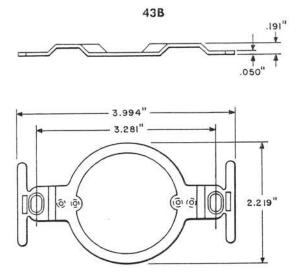
Metal bracket arranged to mount a 47C or D type connecting block or a 108A type apparatus blank in an electrical outlet box. Provided with mounting screws and screws for mounting a connecting block or jack.
