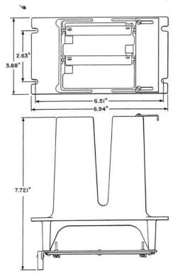
Consists of a die cast metal panel equipped with two 913A Connectors on one side and a terminal panel and two fanning strips on the other side.
