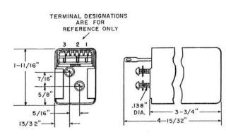
Shell type coils each having a silicon steel core and assembled in a metal case provided with a magnetic shield.
