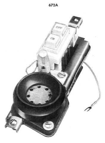
Consists of an AC3 Transmitter Unit, a three transistor feedback amplifier, a volume control, two push button spring contacts, and an associated lamp block assembled on a metal mounting. Overall dimensions are 6 inches long by 1.920 inches wide by 2.730 inches high.
