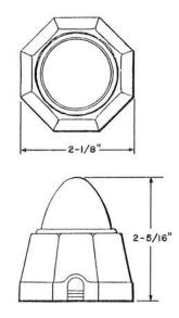
Single lamp indicator equipped with a 358A Electron Tube, in series with a KS-13490L1 (8200 ohm) resistor, and having a clear beehive lens. Housing is of insulating material.
