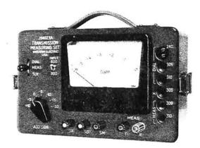
The 23A, B, and C (J94023) type sets have a measurement range from -25 to +10 dbm in the frequency range of 300 to 5000 Hz.
