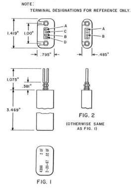
Metallized mylar capacitors potted in synthetic gel in aluminum cans. Minimum capacitance values unless otherwise noted are stamped on end of can.
