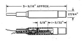
257A: Arranged for jacks with tip springs on the right. Comcode: 100 395 375
