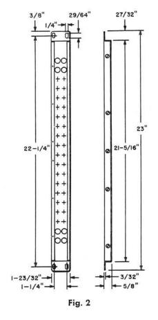
231A: Arranged to mount 218A or similar jacks, backto-back on 5/8-inch vertical and horizontal centers in positions 1 through 32.
