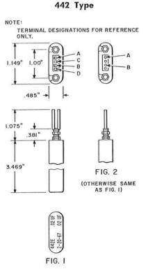
Metallized mylar capacitors potted in synthetic gel in metal cans. Minimum capacitance values are stamped on end of can.
