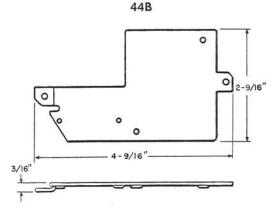
Metal bracket for mounting a number 7 type buzzer and a 152A Capacitor. Mounting screws and two leads for connecting buzzer are furnished.
