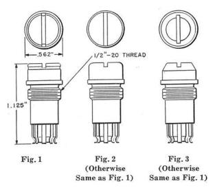
Each unit consists of a metal cap within which is assembled a coil spring and a metal cage containing a pair of protector blocks, as indicated in table, and a fusible alloy spacer.
