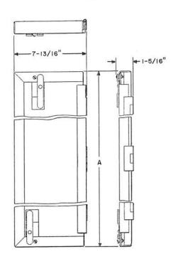
Each consists of a light olive gray enamel finished sheet metal end section arranged for closing the ends of one or a group of intermediate sections. Screws and nuts for fastening to intermediate sections are furnished.
