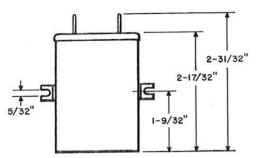
Consists of loading coil and capacitors potted in metal case. Passes frequencies below 3000 Hz and is designed to operate between 600-ohm line and subscriber set.
