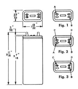
Paper capacitors potted in wax in aluminum cans. Minimum capacitance values unless otherwise noted are stamped on can.
