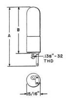
Tungsten filament lamps with a molded base having two soldering terminals. Will mount on relay mounting plates on 1-inch centers and on mounting plates drilled or punched for E, R, or U-type relays.
