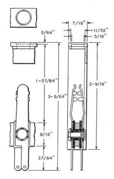
The number 30 Lamp Sockets are strip-mounted and are furnished only on orders for lamp socket mountings.
