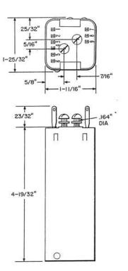
Consists of windings on a silicon steel core, two thermistors, and a resistor potted in a metal can.
