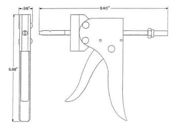
Consists of a metal housing having a hand-grip operating lever that actuates a ratchet rod. Arranged to accommodate a 716A or 716B Tool.
