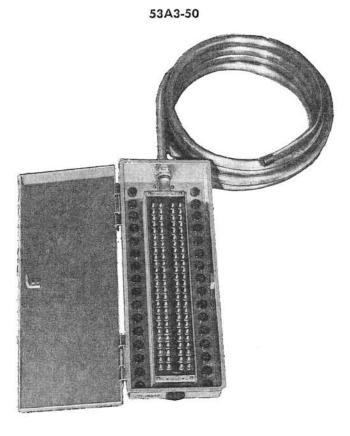
The 53A3-50 Cable Terminal is a 50 pair cable terminal used as an unprotected distribution terminal at locations where there is a heavy concentration of drop or block wires and is intended for wall or pole mounting. Overall dimensions are 22-7/8 inches high by 8-3/16 inches wide by 2-1/2 inches deep.
