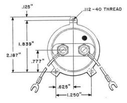
Consists of an AC1 Transmitter Unit equipped with 18-inch long leads and a clamp ring. Mounting screws are furnished. The cord tips are arranged for number 4, 5, or 6 screws.
