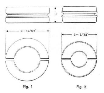
Each consists of two east metal spacers, a clamping ring (shipped loose), and a length of lashing wire (shipped loose). 133A, B, and C: Intended for use with 10A. 12A, 29D type, and 21D type splice cases. See Fig. 1.
