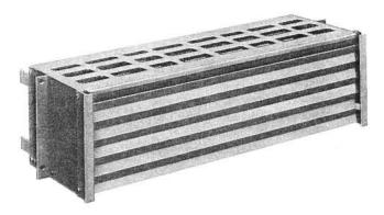
Each consists of a metal housing arranged to mount on a 23 inch wide rack, containing J87270A-1 rectifiers. Overall dimensions are 22.93 inches long by 6.105 inches high by 8.82 inches deep.
