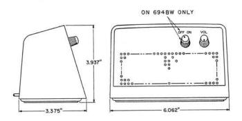
694AW: Consists of a transistorized amplifier and two terminal strips assembled on a printed wiring board, a KS-16881L1 Loud Speaker, an AC1 Transmitter Unit, and a volume control all of which are mounted on a metal base and enclosed in a plastic housing. Provided with a D4BM Cord having the same color as the housing.
