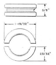
Consists of two cast metal spacers, a metal clamping ring, and a length of lashing wire. The clamping ring and lashing wire are shipped loose.
