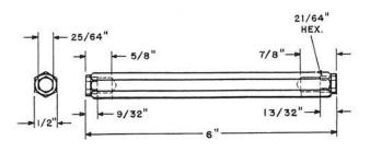
A double socket wrench for use on 21/64 inch and 25/64 inch hexagon nuts on receivers, transmitters, and subscriber set binding posts.
