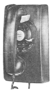
Common battery wall type sets each having a snap-on type cover. Volume of ringer may be changed manually by means of an arm projecting from the underside of the cover. Ringer can be silenced by removing the cover and making a minor adjustment. Overall dimensions with hand set in place are 5-1/2 inches wide by 5-19/32 inches deep by 9-13/16 inches high.
