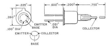
18A: Consists of a pair of N-P-N silicon nonepitaxial mesa transistors, one of which is shown in the illustration. The pair is matched so that the product of the common emitter current gains is in the range of 3,200 to 14,000.
