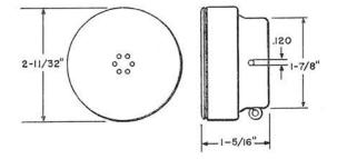
716A: Consists of HA1 Receiver Unit assembled in 11A Receiver Holder which has phenol plastic cap and case having terminal and cording facilities.
