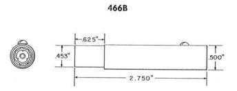
A portable patching jack having coaxially arranged inner and outer contacts. Tested at 1000 and 2000 volts ac. Used with KS-8086 or number 724 cable and with 337A and B and 342A and B Plugs in the type L Carrier Telephone System.
