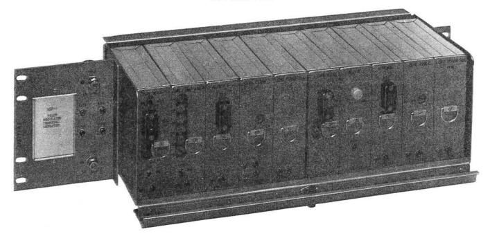
The WLR-5 wideband loop repeater is used to condition loops for wideband data transmission. It provides amplification and continuously adjustable loss equalization to postequalize wideband local loops.
