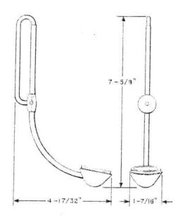
55AW: Consists of a formed tubular metal arm, a stop bar, a terminal block, and a transmitter case arranged for an N1 Transmitter Unit.
