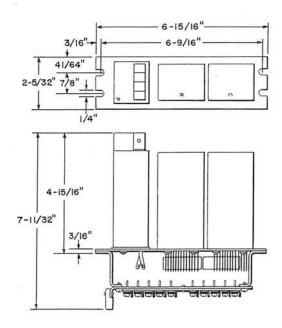
Terminal panel consists of a group of 20 terminals, arranged in 2 rows of 10 each, numbered 1 to 20.
