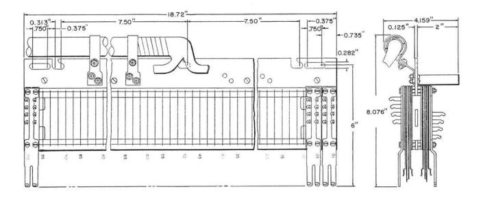
301A1-100: Consists of a 444C Jack equipped with a universally mounted number 24 AWG color-coded plastic insulated stub cable with an aluminum shield, a polyvinyl chloride sheath, and a fanning strip. The stub cable is equipped with a gas plug. Connectors are arranged for 100 pairs of conductors and provide a ready means of opening lines and trunks for testing and other purposes. Mounting screws are furnished.
