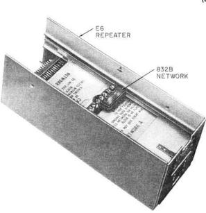
The E6 Repeater is a two-wire voice frequency, transistorized repeater designed to reduce the transmission losses of exchange area trunks. The repeater assembly consists of a shell in which the various networks are mounted.
