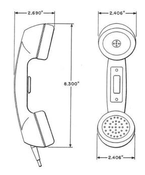
The G10BW is the same as the G10AW except has a single push bar to control both transmitter and receiver simultaneously.
