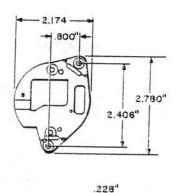
Consists of stamped stainless steel plates used to shockmount a P-type ringer. To be mounted adjacent to a resonator cavity or inside a telephone set housing which has been tuned as a resonator cavity.
