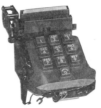
A multifrequency TOUCH-TONE dial having 12 push buttons and a medium gray cover plate. Each of the buttons, when operated, generates a dual frequency signal distinctive to that button. Overall dimensions are 3.480 inches high by 3.421 inches wide by 1.760 inches deep.
