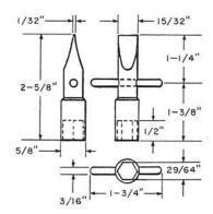
A combination socket wrench and screwdriver for use on number 7 type fuses. Socket engages hexagon nut, 7/16 inch across flats. Comcode: 100 750 546
