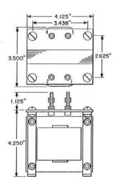
Consists of winding on grain oriented silicon steel core clamped between brackets which provides a means for mounting.
