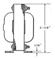
Consists of a winding on a silicon steel core clamped between metal brackets which provide means for mounting.
