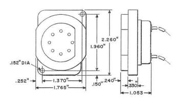
A controlled diaphragm magnetic type transmitter unit. The impedance at 1000 Hz is approximately 300 ohms. The unit is equipped with two black terminal leads approximately 2-1/2 inches long.
