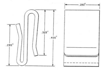
A copper tinned stainless steel spring type adapter. Used to terminate spade tip terminated cords to 66 type quick-clip type connectors.
