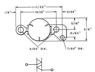
Consists of two 1/2-inch diameter oxidized copper discs in a metal case. Provided with two terminals for electrical connection and also for mounting purposes.
