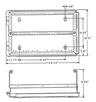
A metal framework assembled on a metal backboard, hinged to permit access to front and rear of apparatus when assembled on this mounting. Provided with six cable rings, six blocks, and screws for mounting the cable rings and blocks.
