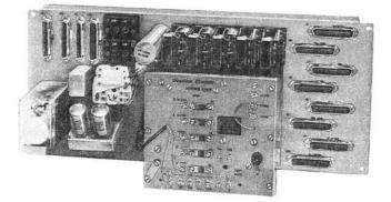
Consists of a power unit, an interrupter, relays, connectors, and pigtail components mounted on a panel. Arranged for relay rack mounting by four 0.32 inch by 0.25 inch holes located on 22.312 inch by 9.00 inch centers.
