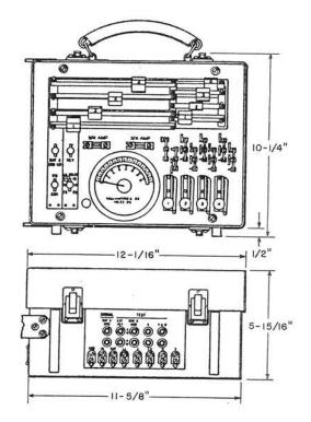
A dc regulating and measuring device intended for use in testing and adjusting relays and other apparatus for which current flow and voltage requirements are specified.
