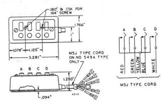
Consists of four nonlocking push button keys mounted in metal boxes. Keys are equipped with white plastic push buttons and provided with an escutcheon plate and designation card.
