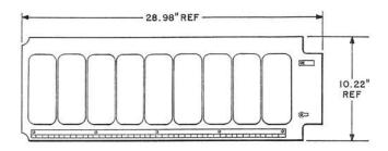
Consists of a fanning strip mounted on a terminal plate assembly 1 inch deep with a six foot AT-7441D Inside Wiring Cable.
