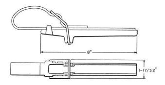
An adjustable strap wrench with a metal handle. Used for tightening and loosening the transmitter and receiver caps of hand sets and for other applications where an adjustable strap wrench can be used.
