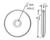
Disposable paper pad intended for use, when required, on the receivers and head sets to provide a comfortable fit. The side of the pad that contacts the ear is covered with six layers of absorbent tissue, five of which may be removed one at a time when the tissue becomes soiled.
