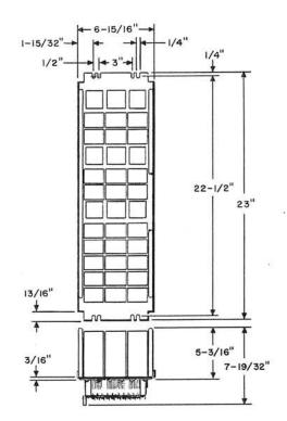
Terminal panel consists of four groups of terminals. Each group has 40 terminals, arranged in 4 rows of 10 each, numbered 1 to 40.
