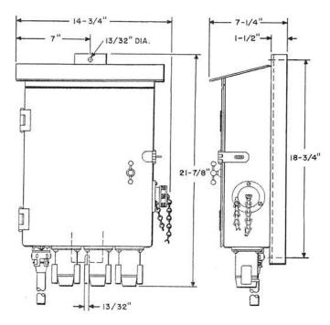
Each consists of a G16B Binding Post Chamber mounted in a weatherproof metal box which is arranged for mounting on a post or pole.
