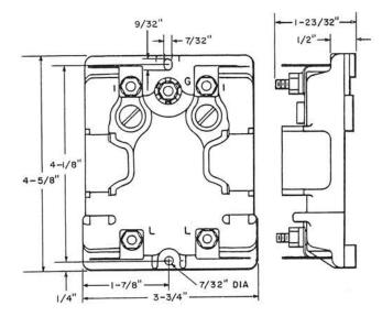
Base of insulating material equipped with two 2A1A Protector Units. Spring assembly, with sufficient current carrying capacity, is included in protector well and makes fuseless operation possible.
