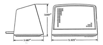
Consists of a permanent magnet dynamic loud speaker mounted on a metal base having a plastic housing, with cord of same color furnished. Has a nominal impedance of 23 ohms at a frequency of 1000 Hz, and an approximate dc resistance of 19 ohms, both exclusive of the cord.
