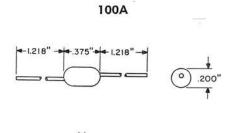
Each consists of two silicon varistor discs encased in resin and equipped with tinned leads. Rated at 10 microamperes in either direction in turn at 0.2 volts dc.
