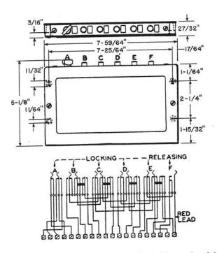
Consists of a key unit and a terminal strip enclosed in a black metal box. The contact springs are strapped to the terminal strip for outside connection. The keys are equipped with five black push buttons and one black turn button.
