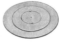
A plastic plate having overall dimensions of 4.500 inches in diameter with a depth of 0.509 inch.
