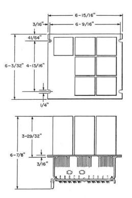
Terminal panel consists of two groups of terminals. Each group has 40 terminals, arranged in 4 rows of 10 each, numbered 1 to 40.
