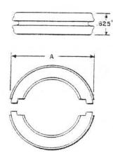
Each consists of two cast metal spacers, a metal elamping ring (shipped loose), and a length of lashing wire (shipped loose).
