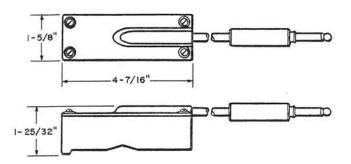
A low impedance test set consisting of an exploring coil enclosed in a cast resin block. A 6-foot cord equipped with a 347A Plug is permanently connected within the block.
