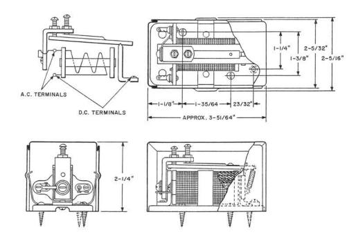
High resistance buzzer equipped with a light olive gray dust cover. Designed to operate on either direct current of 24 volts or alternating ringing current of 16-2/3 cycles. Approximate resistance is 1200 ohms. When mounted on metal surfaces a number 176A-49 Backboard is required and must be ordered separately. Comcode: 100 014 281
