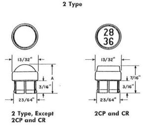
Thick, substantial lenses made from specially selected and treated glass, unless otherwise noted. Lenses are held firmly in place in cap cases by spinning the edges over the lenses. Dimension A is 17/32 inch for the 2BR, 2BS, 2BT, 2EE, 2EF, and 2EG, and 15/32 inch for all other codes.
