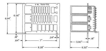
Terminal panel has 80 terminals, arranged in two groups of 40 terminals each. Each group is arranged in 4 rows of 10 terminals each, numbered 1 to 40.
