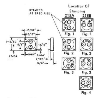
Mounting of black insulating material that will accommodate two jacks.
