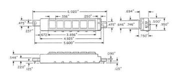
A white molded compound with a plastic appearance which is intended for use in the 3640AW and 3641AW Type Telephone Sets to fill the space reserved for additional keys. The width of the apparatus blank is the same as one of the keys.
