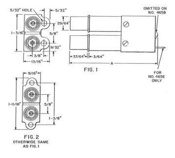
Consists of a pair of coaxial jacks held rigidly in a metal cover. Each jack has an inner contact held in a tubular shield which is the outer contact. The outer contacts of the two jacks are connected together electrically. Jacks are arranged for number 185 and 230A Jack Mountings. Two screws are provided for mounting.
