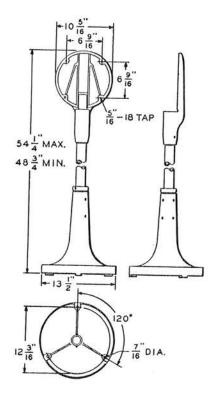
Intended to mount a number 320 type telephone set. The height is adjustable within the limits indicated on the illustration. Black finish. Bolts are furnished for mounting the telephone set to the pedestal.
