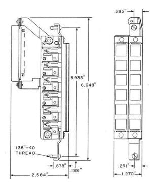
Consists of two molded lamp strips, each containing six lamp sockets equipped with 51A Lamps, and a KS-16672L1 Connector assembled to a metal bracket. Lamp sockets are wired to the connector.
