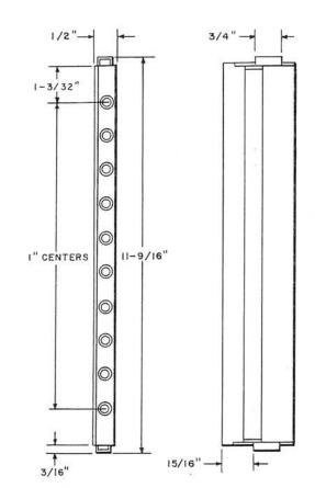
Metal mounting with a face of insulating material that will accommodate 10 jacks. Furnished only on orders for jacks and unnumbered unless otherwise specified on orders. Not furnished partially equipped with jacks. The lower edge is grooved.
