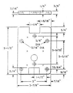
168D-49: Plastic backboard, light olive gray color. Intended to mount a 42A or 44A Connecting Block on uneven or masonry surfaces. See Fig. 1.
