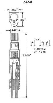
Combination push and turn button key. Pushing button in operates two make contacts, nonlocking. Turning the button operates one make contact, locking.
