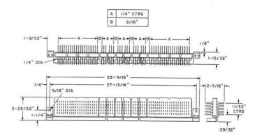
Has five rows of 100 terminals each molded in a cast resin block mounted on a metal angle equipped with a mounting lug and fanning strip. Terminals are arranged for mechanically wrapped connections.
