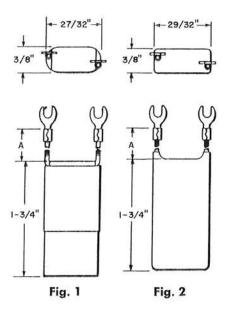
Plastic film wax impregnated capacitors each having an enveloping gray finish, except 198C which is wrapped with tape.
