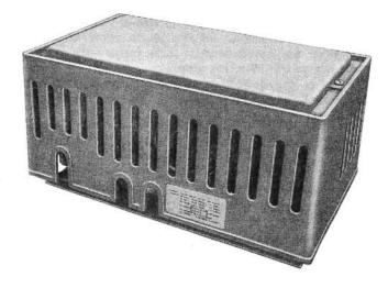
A packaged power supply without battery reserve. Output connections are made through an Amphenol connector type 26-4200-8S which is designed to mate with Amphenol connector type 26-4100-8P. Arranged to mount in key telephone system cabinets.
