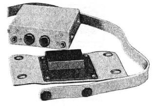
A portable amplifier, consisting of three stages of audio frequency amplification with tuned input and output transformers. Input and output jacks and a gain control are provided in addition to a switch for selecting high or low input impedance.
