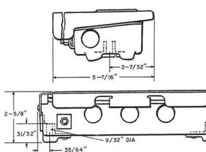
Consists of a cast metal housing having a hinged metal cover and containing twelve 2A1A Protector Units, six pairs of terminals, and two terminals for ringing ground connections. Also equipped with a clamp for connecting a ground wire to the housing to provide protector ground. Can be mounted on poles, crossarms, or walls by means of screws which are not furnished.
