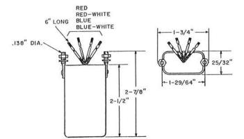
Consists of a toroidal type coil having a permalloy powder core, and a capacitor potted in a metal case. The capacitor (5100 mmf) is connected between terminal leads red and blue-white.
