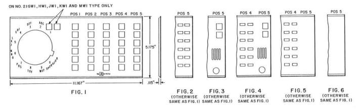
Clear plastic face plates, each containing openings to accommodate a dial, key buttons, and/or a transmitter, on associated telephone sets. Provided with three face mats colored silver, gold, and a color coordinated with the telephone set color.
