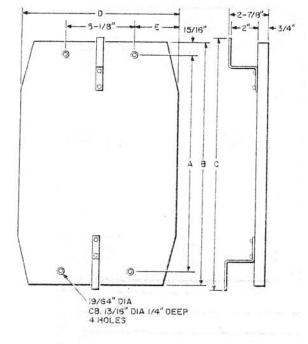
83A: Wooden backboard provided with distributing ring at each end. For mounting binding post chambers or connecting blocks in L-type cable terminal sections. Part of LA16 Cable Terminal Section.
