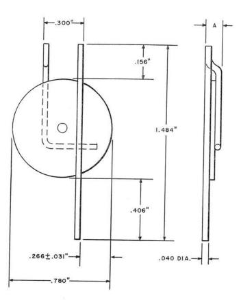
Each consists of a .780 inch diameter silicon carbide disc with metalized surfaces provided with a terminal on each surface for electrical connection.
