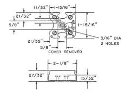
A block of insulating material equipped with four screw terminals, associated screws and washers, and a removable plastic cover.
