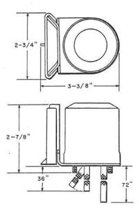
Each consists of three carbon electrodes, having .020 inch gaps, mounted on a porcelain base and enclosed in a metal case.
