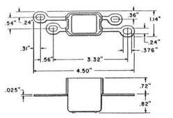
Plastic container provided with terminals which are also used for mounting on terminal distribution blocks.
