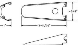
For use as a lever in removing number 275 and 276 type relays from their sockets. Has wedge projections at one end which are intended to be inserted between the base of the relay and the socket.
