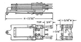
"This dimension varies according to the number of contact springs and winding terminals on the individual relays.
