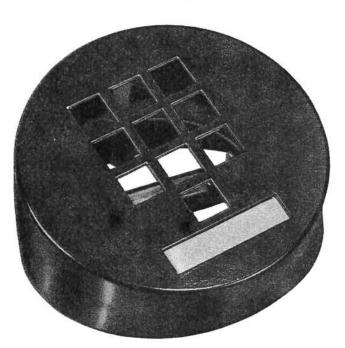
Consists of a molded plastic housing, a dial adapter, and a connecting block for terminating the dial leads. Overall dimensions are approximately 4.500 inches in diameter by 3.275 inches high.
