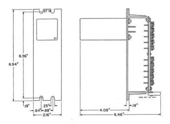
Terminal panel has 20 terminals arranged in 10 rows of 2 terminals each, numbered 1 to 20.
