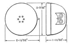
Consists of 12A Receiver Holder and HC3 Receiver Unit which will accommodate cords with number 130 Cord Tips.
