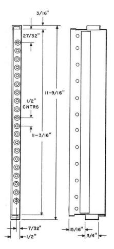
Metal mounting with a hard rubber face that will accommodate 20 jacks. Furnished unnumbered unless otherwise specified on order. The lower edge is grooved, and spotted unless specified.
