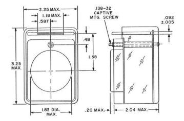
The KS-19175L1 Interrupter is an ac motor driven spring and cam type interrupter having five sets of contacts with various interrupting intervals. It consists of
