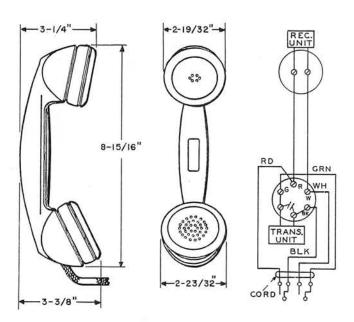
Black finished hand set consisting of an F1 Transmitter Unit, LA3 Receiver Unit, F2W-3 Hand Set Handle, and an H4CA-3 Cord with a 289B Plug.
