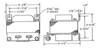
Each consists of a winding on a silicon steel core clamped between metal brackets which provide means for mounting.
