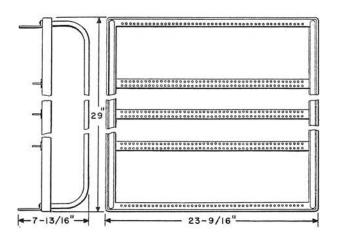
Metal frame arranged to mount four rows of 200 type key telephone units or similar type units or 12 mounting plates, 2 inches high and 23 inches long, or a combination of units and plates. Can be modified to hold 13 mounting plates by removing two of the horizontal T-section mounting bars. Four supports and eight screws are furnished. Two of these supports are assembled in the top and two in the bottom to protect the terminals in the key telephone units.
