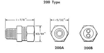
Each consists of a coupling, hexagon cap, rubber bushing, and compression washers.
