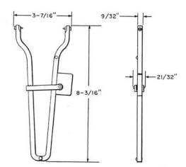
Intended for use in removing and replacing transmitters, receivers, and various parts on E1B type hand sets.
