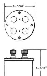
A thermoelectric couple in which the junction of two dissimilar metals is heated by passing a current through a resistance wire to the midpoint of which the junction is attached. These elements are enclosed in a highly evacuated glass bulb which is packed in cotton and mounted in a container of insulating material. Four terminals are provided at one end, two (marked H) for connection to the heater element and two (marked G) for connection to the couple element.
