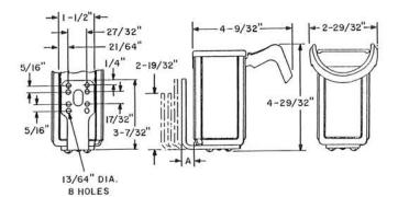
Hand set mountings equipped with a bracket designed to permit adjustment of the mounting to various lengths of desk top overhang. The bracket also permits the mounting to be secured for the hand set to hang at either side or in front of the mounting. Dimension A is adjustable to four lengths: 17/32 inch, 27/32 inch, 1-5/32inches, and 1-15/32 inches.
