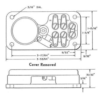
Consists of an inductor and five screw type terminals assembled on a base of insulating material and equipped with a 101A type cover. 1542A-49 is light olive gray. 1542A-50 is ivory.
