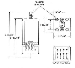
Consists of 10 small paper units potted in metal can with metal cover. One side of each unit is connected to common terminal; other side is connected to one of 10 terminals.
