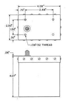
Consists of windings on a silicon steel core having magnetic shunts potted and assembled in a metal can which provides magnetic shielding.
