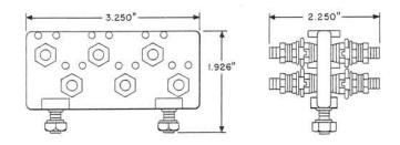
Consists of an injection molded block equipped with six pairs of binding posts mounted back to back with three pairs on each surface of the block. Each binding post is provided with nuts, flat washers, and insulation crushing washers to permit making cable terminations without removing insulation.
