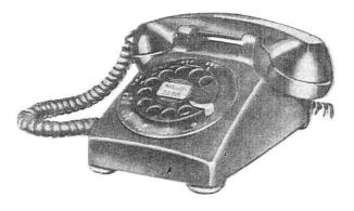
Common battery desk type that provides improved performance transmission, dialing, and ringing functions. These gains can be used either for extension of range of operations from central office or increased use of fine gauge cable conductors. Volume of the ringer may be varied in four steps. By removing the housing and making a minor adjustment, the ringer can be silenced.
