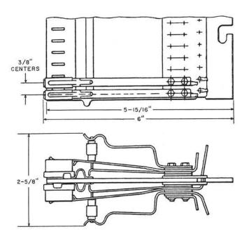
For use on main distributing frames. Overall length is 18-23/32 inches for the C50A and 19-15/32 inches for the C52A.
