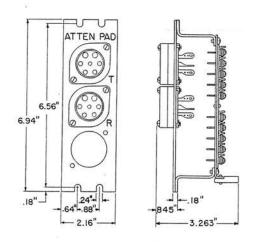
Terminal panel has 20 terminals arranged in 2 rows of 10 terminals each, numbered 1 to 20.
