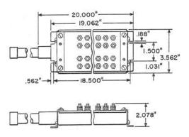
Consists of a sheet metal chamber having an insulating panel equipped with 100 binding posts.
