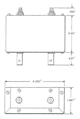
Consists of 237A Resistors mounted on two rotary switches enclosed in a metal can. Equipped with two 217A Connectors for input and output connections.
