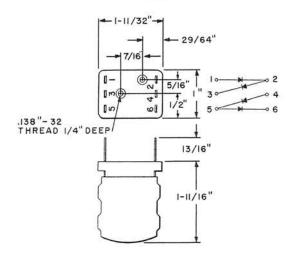
Consists of twenty-four 3/16 inch diameter oxidized copper discs in a block of insulating material.
