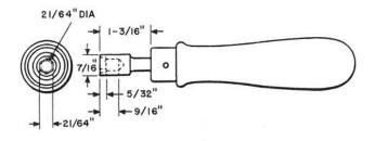
A socket wrench for use on armature adjusting nuts of relays and clamping and mounting nuts of number 114 and similar type relays.
