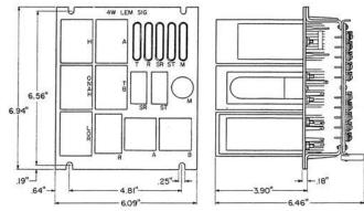
Terminal panel has 80 terminals, arranged in 2 groups of 40 terminals each. Each group is arranged in 4 rows of 10 terminals each, numbered 1 to 40.
