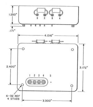
Consists of two tuned circuits, each consisting of a toroidal inductor on a permalloy powder core and one or more polystyrene capacitors potted in a hermetically sealed metal can. Provided with a terminal for grounding the can and four hermetically sealed terminals on the bottom of the can for use on printed wiring boards. May come equipped with trimming capacitors mounted on four hermetically sealed auxiliary terminals located on the side of the can.
