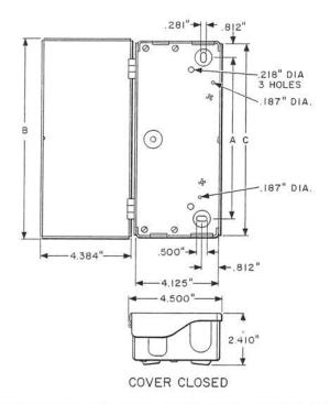
A sheet metal box with a hinged cover, having a light olive gray enamel finish. Provided with knockouts in each end for cable and wire entrance. Also provided with one 8A Distributing Ring and screws for mounting terminal block or adapter and the distributing ring.
