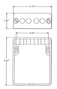
A mounting of insulating material, arranged to mount four 223A or similar type jacks. When so equipped, will accommodate two 289B or similar type plugs.
