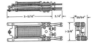
\*This dimension varies according to the number of contact springs and winding terminals on the individual relays. 3-5/16
