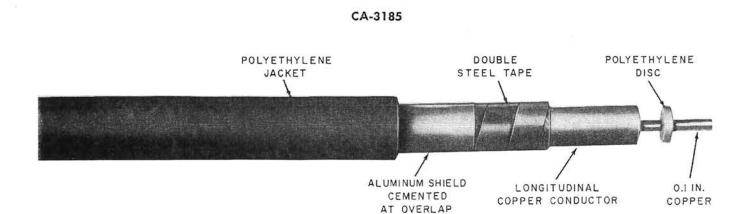
A single coaxial cable manufactured for high frequency transmission.
