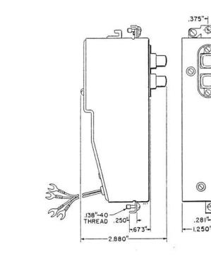
Consists of twelve nonlocking plunger-operated spring combinations, a connector, and two ground strips assembled on a mounting. The ground strips are located under the two rows of spring combinations and are connected by means of a removable strip. An 8-inch long flexible lead, terminated in a cord tip arranged for a number 4, 5 or 6 screw, is connected to the ground strips. Overall dimensions are approximately 6-5/8 inches long by 1-1/4 inches wide by 2-7/8 inches deep.
