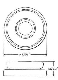
A carbon type transmitter unit intended to mount in a 55AW Transmitter Arm. It forms a part of the number 52 type head telephone sets.
