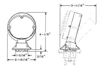
Mounts number 6 type dials. Has a removable cover plate providing access to the dial terminals. The connections from the dial to the hand set mounting pass through the inside of the base.
