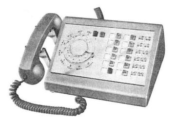
All purpose, jack equipped, large capacity three-position key telephone set with overall dimensions of 12.5 inches wide by 8.125 inches deep by 4.226 inches high.
