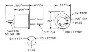
Each is an N-P-N silicon junction transistor assembled in a hermetically sealed metal can.
