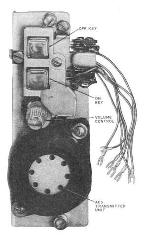
Consists of an AC3 Transmitter Unit, a three transistor feedback amplifier, a volume control, two push button operated spring contacts, and an associated lamp block assembled on a metal mounting. Terminated with seven leads equipped with cord tips for connection to associated circuitry.
