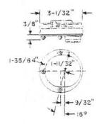
Each consists of a soft rubber gasket provided with three eyelets and three screws for mounting, except 59D which is made of semihard rubber and is provided with only two eyelets (those on the vertical center line of the illustration for 59B and C) and two mounting screws. All are black with the exception of 59C which is gray.
