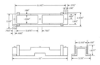
Consists of a molded plastic "stand-off" bracket for mounting 66M type connecting blocks away from flat surfaces so that cables can be stored behind the connecting block. This cable space accommodates three layers of four 25 pair inside wiring cable. The bracket is attached to a wall by means of mounting lugs having slotted holes to accommodate screws or bolts. The connecting block is attached to the bracket by means of a molded in "snap-on" arm.
