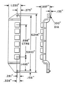
A molded opaque white plastic apparatus blank. Mounted by means of two extruded dowels.
