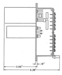
Terminal panel has 20 terminals, arranged in 2 rows of 10 each, numbered 1 to 20.
