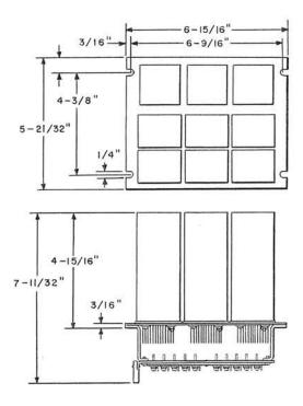
Terminal panel consists of two groups of terminals. One group has 40 terminals, arranged in 4 rows of 10 each, numbered 1 to 40; the other group has 20 terminals, arranged in 2 rows of 10 each, numbered 1 to 20.
