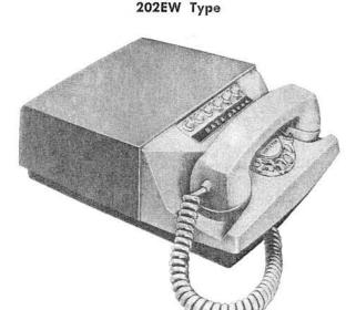
The 202EW type Data Set is an FM transmitting data terminal integrated with a rotary dial telephone set in a two-tone gray plastic housing. Provides normal point-topoint transmission of voice or of serial digital information at data transmission rates up to 1200 bauds on the switched network or up to 1800 bauds on some private line facilities. Designated for voltage signal interface.
