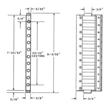
Metal mounting with a hard rubber face that will accommodate 10 jacks. Furnished only on orders for jacks and unnumbered unless otherwise specified. Not furnished partially equipped with jacks. The lower edge is grooved.
