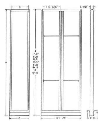
A common systems channel-type relay rack with floor angle and detachable guard rails. Groups 1 through 6 and 28 and 29 cover the various relay racks. Groups 7 through 16 and 19 through 27 are optional details which must be ordered as required. The groups required as described below must be specified on the order.
