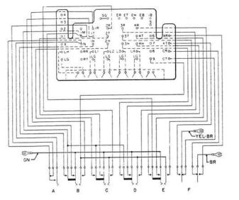
at the terminal strip, the positions can be converted in the field to Pickup (Locking). The releasing plungers, which are nonlocking, and the locking plungers will release any plunger that is locked. The nonlocking plungers and the turn button will not release locked plungers, unless otherwise indicated by footnote. Operation of any two or more locking plungers simultaneously is prevented by means of a lockout feature, unless otherwise indicated by footnote.
