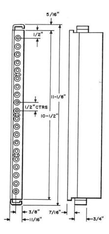
Metal mounting with a hard rubber face that will accommodate 20 jacks. Furnished unnumbered unless otherwise specified on order. The lower edge is grooved and spotted unless otherwise specified.
