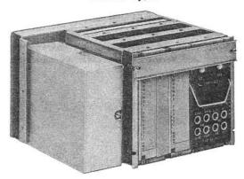
Provides line interfacing, test features, and interconnection arrangements for the component units of wideband data stations using the Data Set 303 type.
