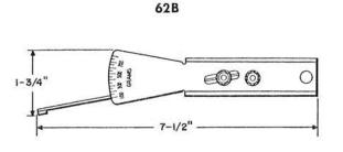
Consists of handle on which indicating spring is mounted. Both sides of handle have scale graduated in 50 gram steps from 0 to 700 grams.
