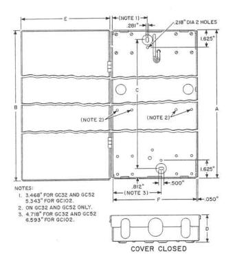
A sheet metal box with a hinged cover, having a light olive gray enamel finish. Provided with knockouts in each end for cable entrance and in each end and one side for wire entrance. Also provided with one 8A Distributing Ring. Screws are provided for mounting terminal block or adapters.
