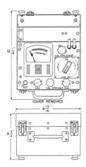
Consists of component apparatus assembled on a metal panel and enclosed in a metal box having a removable cover. A W6E Cord is provided. Contains a compartment for dry cells and another for storing the cords and plugs.
