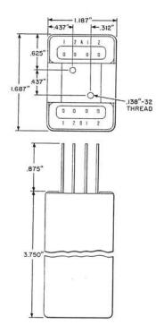
A metal container arranged to contain two 652, 658, 659, 641, 642, or 643 Loading Coils or 1574A, 1574B, or 1613A Inductors. The quantity and code numbers of the coils or inductors must be specified in the order. Individual cases cannot contain mixed codes.
