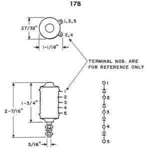
Oxidized copper disc type varistor with an enveloping lacquer finish. Consists of sixteen 3/4-inch diameter discs arranged electrically to form a bridge with four discs in series per arm. At an ambient temperature not exceeding 105° F, it is designed to have a maximum continuous output per arm of .075 amperes dc and a potential per arm of 12 volts dc.
