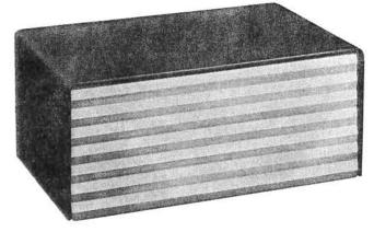
Data Set 402DW3: The receiver of a medium-speed, binary parallel data transmitter. Receives signals from the transmitting component of the system and delivers any number of binary data levels up to 8 at any speed up to 75 characters per second. Timing information is also received and delivered. A nonsimultaneous answer-back feature is provided at a maximum operating speed of 20 two-bit characters per second.
