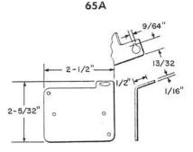
Metal bracket for mounting a number 7 type buzzer or a KS-8109 type buzzer in a 630DW type and similar multibutton type telephone sets. Mounting screws are furnished and also insulated washers are furnished for mounting a KS-8109 type buzzer.
