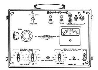
A portable test set available in two forms: as an ac operated oscillator and detector or an ac operated oscillator only. It can be adapted for mounting in 19- or 23-inch equipment racks. Dimensions excluding cover are 17 inches long by 12 inches high by 8 inches deep. Weight is 37 pounds. Operates on 115 volts, 60 Hz.
