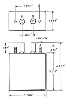
Consists of component apparatus mounted on a printed wiring board and assembled in a metal case. Terminated in two 217A Terminals.
