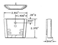
Two-piece metal bracket for mounting 101B Wire Terminal. Intended for pole or crossarm mounting of terminals so that removal and replacement will not interrupt service. Mounting hardware is furnished.
