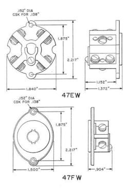
Each consists of a block of insulating material equipped with screw terminals. Arranged for a mounting cord having either a winged type stay band or an S-hook. Mounting screws are furnished.
