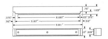
A wooden mounting strip equipped with a black finished metal retaining strip and transparent face strip. Arranged to mount a strip of printed figures under the face strip. Will mount with number 114, 141, and 142 Jack Mountings.
