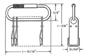
Consists of 100A through 100H and 101A through 101E Gauges assembled on a holding ring.
