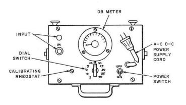
A test set consisting of a three-stage negative feedback amplifier and a rectified-type meter mounted on a panel chassis and enclosed in a metal box. Overall dimensions are 10-7/8 inches by 8-1/8 inches wide by 8-5/16 inches deep with cover.
