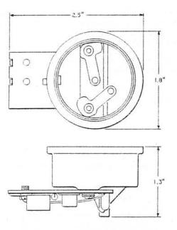
A single-stage transistor amplifier used to amplify telephone set transmitter audio output. Designed to be used in the same manner as 238A amplifier except that it incorporates a polarity guard which permits it to be used where the line is subject to polarity reversals.
