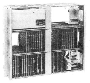
The Data Set 205CW2 is a four-phase modem designed to be used primarily as a terminal station for full period service on either two-wire or four-wire private lines.
