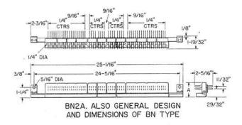
Each has 80 terminals per row molded in cast resin blocks mounted on a metal angle equipped with mounting lugs and provided with a fanning strip. Terminals are arranged for mechanically wrapped connections.
