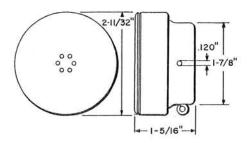
Black plastic case and cap arranged for HA type receiver unit. Forms a part of 716A, B, or C Receiver. Provisions are made for attachment of 11A Headband.
