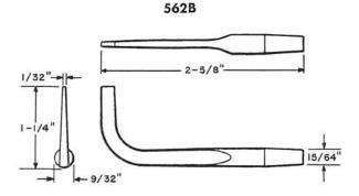
Used in checking the stud gaps of U, Y, and UA type relays.
