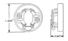
Controlled diaphragm magnetic receiver units.
