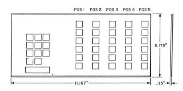
Clear plastic, nonglare type face plates each containing openings to accommodate a dial, key buttons and/or a transmitter, on associated telephone sets.
