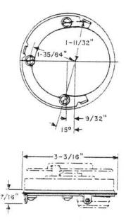
Consists of a metal plate with three mounting lugs, a shield, a 59B Dial Adapter, and the necessary mounting screws.
