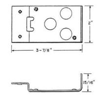
Metal bracket for mounting number 7 type buzzer and a 152A Capacitor. Mounting screws and two leads for connecting buzzers are furnished.
