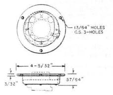
Consists of a black finished flanged metal cup, designed to mount number 2, 4, and 5 type dials, and a black finished metal plate which mounts over the flange of the cup. Screws are furnished for mounting the dial in the dial adapter and for mounting the dial adapter.
