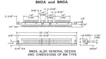
Each has 80 terminals per row molded in cast resin blocks mounted on a metal angle equipped with mounting lugs and provided with fanning strips. The terminals are arranged for mechanically wrapped connections.
