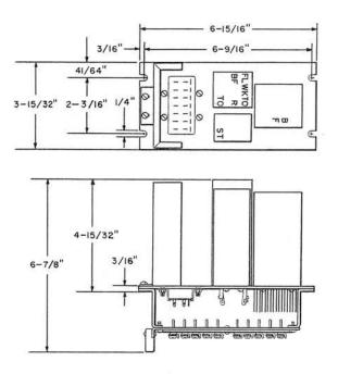
Terminal panel consists of a group of 40 terminals, arranged in 4 rows of 10 each, numbered 1 to 40.
