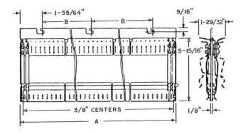
C50 and C52: Consists of a metal plate equipped with springs for holding number 28 and 29 Protector Blocks and 76A Heat Coils. The protector blocks and heat coils do not form a part of the protector mounting. Arranged for pairs of wires as indicated below. Part of C50A and C52A Protectors respectively. Mounting screws are furnished. For use on main distributing frames.
