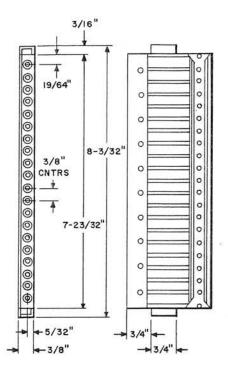
Metal mounting with a hard rubber face that will accommodate 20 jacks. Furnished unnumbered unless otherwise specified on order. The lower edge is grooved, and spotted unless otherwise specified.
