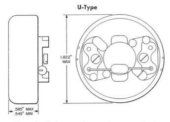
Composite diaphragm, ring armature, magnetic type receiver unit with screw terminals.
