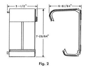
Metal cases, pearl-gray wrinkle enamel finish. Provided with two flat fillister head machine screws for assembly to associated apparatus cases. Intended for use with 705B and 706B Apparatus Cases, respectively, at control centers in connection with air defense systems.
