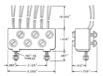
Consists of a cast resin terminal block equipped with six leads, three pairs of binding posts, and six 2A1A Protector Units. Provides facilities for protecting three stations and terminating service wire.
