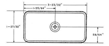
A metal cover furnished in colors listed in table and equipped with a captive mounting screw. Color must be specified on order.
