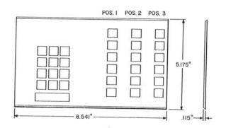
Clear plastic, nonglare type face plates, each containing openings to accommodate a dial and key buttons on associated telephone sets.
