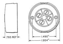
A nonflush type consisting of a block of plastic insulating material containing four intermeshed coil spring contacts.
