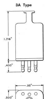
Each unit consists of a five terminal base assembled in a housing of insulating material of color indicated in table. Also contains protector blocks and fusible metal alloy spacers.
