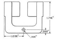
Each consists of a metal spring clamp equipped with a mounting screw.
