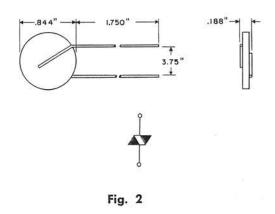
Each consists of a 3/4-inch diameter silicon carbide varistor disc having a coating of insulating material and equipped with tinned leads.
