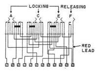
Consists of a key unit and a terminal strip enclosed in a black metal box. The contact springs are strapped to the terminal strip for outside connection. The keys are equipped with black push buttons. The box may be reversed with respect to the key assembly to permit mounting on either the right or left side of a desk or table. The cover is provided with two holes for cable entrance and is attached to the box with screws.
