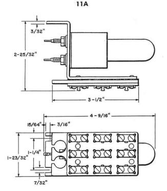
Arranged to mount in a number 105BW Apparatus Box. Requires angle type P-37B204 Bracket for installation on 16C Apparatus Mounting or when unit is relay rack mounted.
