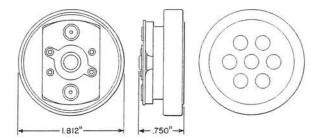
A controlled diaphragm magnetic type receiver unit equipped with varistors to limit the voltage applied to the receiver units and thereby limit acoustic outputs and protect the magnets against demagnetization. HA11 is moisture resistant.
