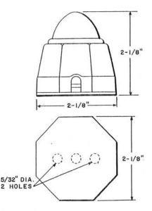
Single lamp indicator equipped with a beehive lens colored as indicated below. Housing is of insulating material and has a light olive gray finish.
