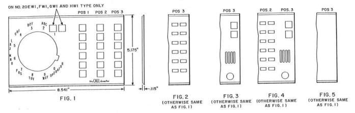
Clear nonglare plastic face plates each containing openings to accommodate a dial, key buttons and/or a transmitter, and switch knobs when specified, on associated telephone sets or consoles.
