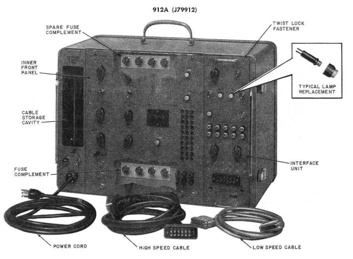
The 912A Wideband Data Test Set is used to test wideband data stations or sets which operate in the range of 9 to 2000 kilobits per second. The test set, designed to be either portable or fixed, determines error rates, tests all interface functions of a wideband data set or station, makes margin tests of received nonsynchronous data and can test low-speed Data Sets 400BW which may be associated with a wideband data station.
