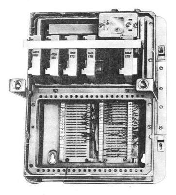
The factory prewired capacity of these units is a total of six circuits. This may be a combination of lines (central office or PBX) and manual intercom. An additional two lines may be added by inserting a 259A Key Telephone Unit, which if required must be ordered separately.
