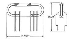
185A: Consists of one each of the 186A through 186E gauges, assembled on a metal key ring.
