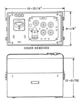
96A: A portable test set consisting of a voltmeter and Wheatstone bridge units, with associated apparatus for supplying dc and ac bridge potentials. It is mounted on a metal panel and enclosed in a metal case provided with a removable cover and a carrying strap. Contains a compartment for the batteries and one for storing the cord and battery leads.
