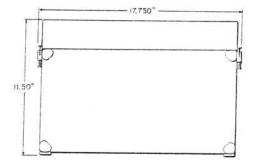
Consists essentially of an amplifier, a meter circuit, and two oscillators mounted on a chassis assembly and metal panel. Enclosed in a metal case having a removable cover. Contains a compartment for batteries and one for storing a receiver and cord. The chassis is equipped with three sockets for storing spare electron tubes which are not furnished and if desired must be ordered separately.
