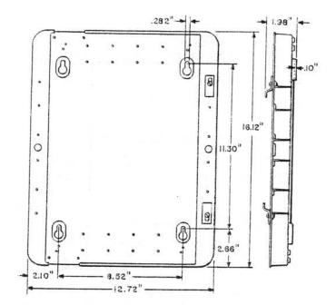
Die cast metal backboard, provided with three cable rings, four blocks, and screws for mounting cable rings and blocks.
