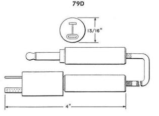
This test set consists of an exploring coil enclosed in a metal case equipped with a handle and a P2AS Cord equipped with a 347B Plug.
