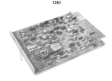
Consists of component apparatus mounted on a printed wiring board terminated in printed wiring terminals. Arranged to be inserted into a 927A Connector.
