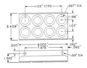
Aluminum brackets equipped with rubber grommets, each of which will accommodate a 25-pair binder group.
