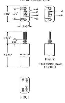
Metallized mylar capacitors potted in synthetic gel in aluminum cans. Minimum capacitance values are stamped on end of can.
