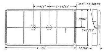
A plastic cover furnished in colors listed in table and equipped with a captive mounting screw and a screw for cord attachment. Color must be specified on order.
