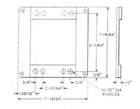
A galvanized welded steel frame. Used for mounting a number 320 type telephone set. Bolts are furnished to mount the telephone set to the backboard.
