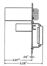
Apparatus mounted on plate is wired to a KS-16672L1 Connector which has 50 contacts arranged in 2 rows of 25 each, numbered 1 to 50.
