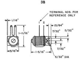
Oxidized copper disc type varistor with an enveloping lacquer finish. Has two parallel opposing arms each consisting of two 3/4 inch discs. Provided with mounting screws.
