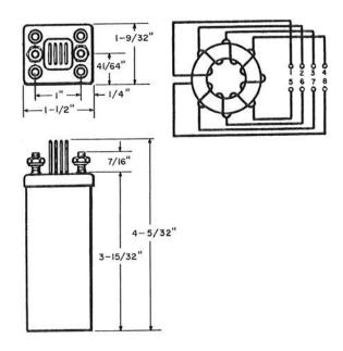
Toroidal type coils having permalloy core; enclosed in metal case. Closest recommended mounting centers are 1-9/16 inches by 1-3/8 inches.
