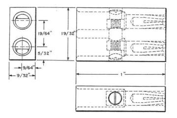
A block of black insulating material provided with two metal sleeves arranged at one end to be attached to an L4T Cord and at the other end to connect to a number 29 Cord Tip by means of plug connections.
