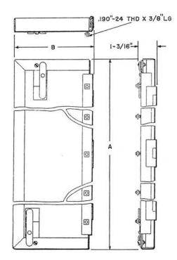
Each consists of a light gray enamel finished sheet metal end section arranged for closing the ends of one or a group of intermediate sections. Bolts and nuts for fastening to intermediate sections are furnished.
