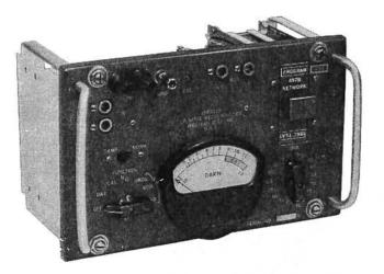
The 3B is a compact, transistorized, rack mounted noise measuring set. The set measures noise in dbrn on message and program circuits. It has both dynamic and frequency characteristics which make its readings comparable to the response of the human ear.
