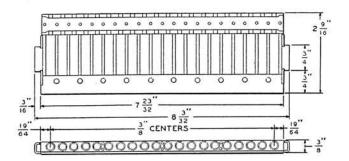
Consist of a metal mounting plate with a face of black insulating material and mounting, insulating, and clamping strips. Arranged to accommodate 20 jacks. Furnished only on orders for jacks and unnumbered unless otherwise specified. Not furnished partially equipped with jacks.
