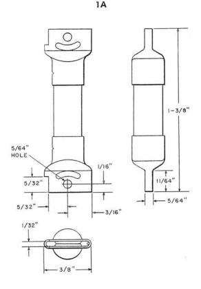
Consists of a circuit element, having a negative temperature coefficient of resistivity, in a glass envelope enclosed in a fiber tube with metal end caps. The thermistor is designed to act as a time delay element in circuits to delay relay operation. With the nominal resistance at 77° F with 60,000 ohms zero current and 450 ohms maximum current, the maximum continuous current is .015 ampere for ac only. Temperature coefficient at 77° F is -1.7 percent per degree F.
