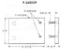
A metal adapter used to mount 19-inch mounting plates on 23-inch span gates and relay racks.
