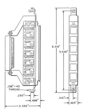
Consists of a molded lamp strip containing six lamp sockets, which are arranged for 51A or 52A Lamps, and a KS-16672L1 Connector assembled on a metal bracket.
