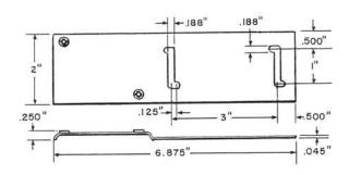
Metal bracket for mounting a number 7 type buzzer on a number 168 type backboard. Mounting screws are furnished.
