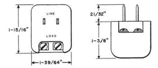
Consists of windings on a silicon steel core, encapsulated in a cast resin case. Available in light olive gray (-49) and ivory (-50).
