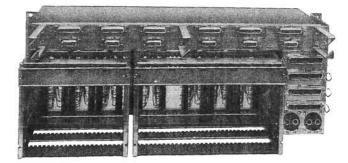
Consists of a 58A Apparatus Mounting, a 59B Apparatus Mounting, 927B Connectors, KS-16786L4 Connectors, KS-19078L1 and L2 Connectors; and 225A Jacks mounted and wired on a panel. Arranged for relay rack mounting by four 0.32 inch by 0.26 inch holes located on 22.312 inch by 7.00 inch centers. Overall dimensions are approximately 23.00 inches long by 7.96 inches high by 8.90 inches deep.
