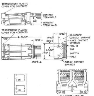
ENLARGED VIEW OF CONTACT END OF AKI WITH COVER REMOVED The AK type relays are generally the same as the AF type, except they are designed to mount interchangeably with the AF type and there are two independent relay units. To effect a space saving, they may be used as a substitute for two AF type relays, each of which has a single winding coil and five or less sets of contacts.
