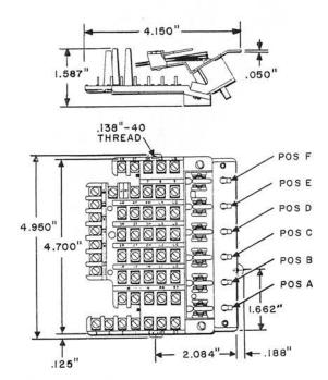
Mechanically locking keys consisting of six spring combinations which are plunger operated and wired to a terminal strip.
