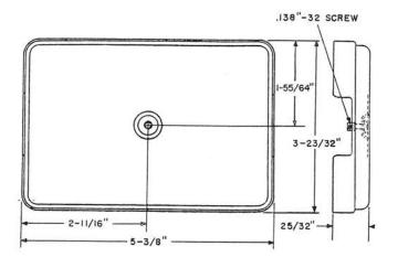
A metal cover furnished in colors listed in table and equipped with a captive mounting screw and a screw for cord attachments. Color must be specified in order.
