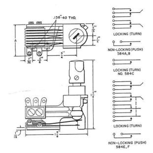
Combination turn and push button type key. Push button can be operated with turn button in either position.
