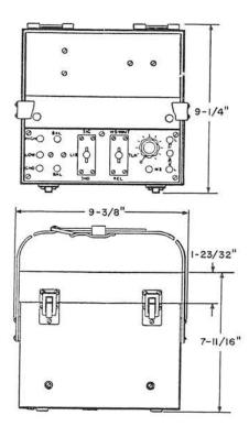
A portable battery operated electron tube oscillator for use by cable splicers on exchange and toll cable for identifying cable wires and other tone testing purposes. Trays for batteries and storage for splicer's talking set (52EW Head Telephone Set) is provided in the case.
