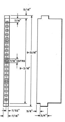
Hard rubber mounting that will accommodate 20 jacks. Furnished unnumbered unless otherwise specified on order. The lower edge is grooved, and spotted unless otherwise specified.
