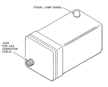
Provides for automatic connections of either one or two Central Office or PBX lines.
