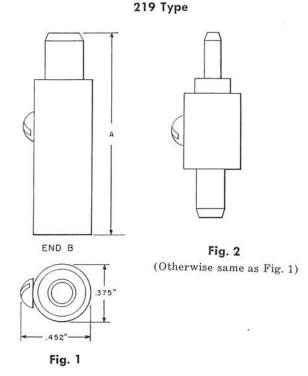
219A: A combination cable termination or cable connector. When used for cable termination, a 724A or 730A Cable is connected to the appropriate terminal and a resistor (not furnished) is soldered from the wire to the outer surface of the unused cable terminal. A sleeve is then positioned so its longer end will be over the resistor side of the connector.
