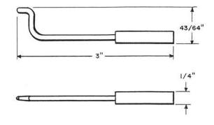
Used in adjusting armature and contact air gaps on polarized relays of number 206 and 215 types.
