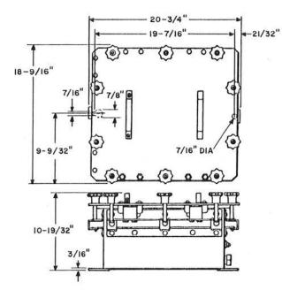
Watertight sheet metal case with removable hinged cover so arranged that by relocating the hinges it will swing open from either the right or left side. Mounts in a manhole or cable vault.
