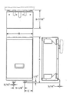
Each consists of a sheet metal intermediate section and door which have a light olive gray finish. Knockouts are provided in top and bottom of details for bringing in cables or wires. Screws and washers for mounting terminal blocks or backboards, and screws and nuts for fastening sections together are furnished.
