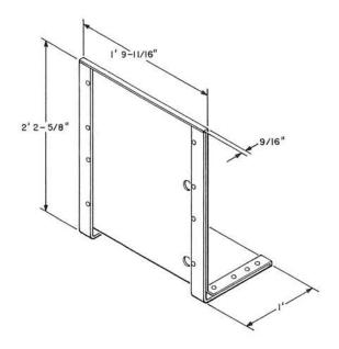
A metal stand which consists of two supports and a cover having a light olive gray enamel finish. Stand has capacity for two cabinets. Screws for mounting are furnished.
