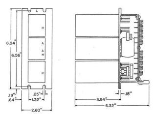
Terminal panel has 30 terminals, arranged in 3 rows of 10 terminals each, numbered 1 to 30.
