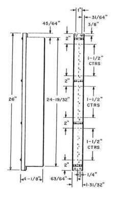
Metal plate drilled to mount 15 U- or Y-type relays on centers as shown with the U-type relay having no more than three winding terminals at either the top or bottom and the Y-type having no more than two winding terminals at either the top or bottom.
