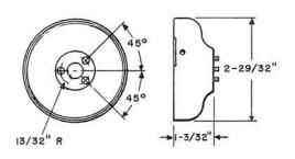
Consists of a black finished metal mounting for mounting on residence system sets and similar apparatus. Mounting screws are furnished.
