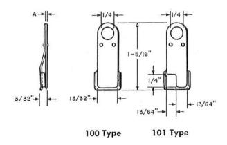
Components of 99A Gauge. Individual gauges of thickness are indicated in table.
