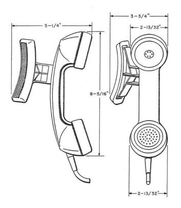
Consists of a T1 Transmitter Unit, a U3 Receiver Unit, and an H4CJ Cord. Equipped with a removable support having a removable pad for holding hand set on the shoulder. The shoulder support, which is shipped loose, may be assembled to the hand set for use on either the left or the right shoulder. The illustration shows the shoulder support assembled to the hand set for use on the left shoulder. Available in colors shown in the table.
