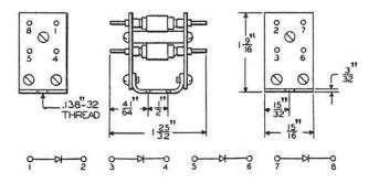
Multiple semiconductor type, consists of four arms, each arm having a single number 405 type diode, assembled between terminal plates which are supported by a metal bracket containing two mounting holes.
