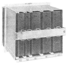
Consists of a metal casing equipped with two 906E and three 908C connectors, a terminal panel, and five circuit packs.
