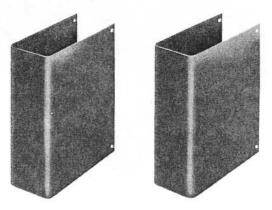
ED-95023-70, Groups 4 and 5, consist of two baked gray enamel finished metal covers used to conceal exposed portion of metal stand where appearance is important. Each cover has four 0.191 inch diameter mounting holes and eight number 8-32 round head machine screws are furnished with each group. The group required must be specified on the order.
