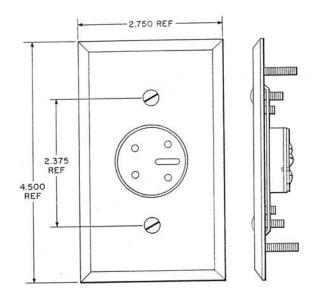
Consists of a 548A type jack, a 43A Bracket, and a flush-type cover plate arranged for mounting in an electrical outlet box.
