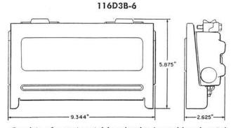
Consists of a cast metal housing having a hinged metal cover and containing a 57A2B-6 Connecting Block. Also equipped with a clamp for connecting a ground wire to the housing to provide protector ground.
