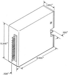
Consists of wire strapping mounted on a printed wiring board and assembled into a metal can. Terminated in a
