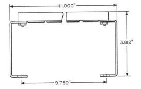
An aluminum bracket equipped with 16 rubber grommets, each of which will accommodate a 25-pair binder group. Also equipped with two aluminum mounting supports. Mounting screws and a single pair wire terminal are furnished.
