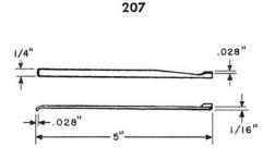
An offset screwdriver used with the number 206 Tool for adjusting the screws holding the springs on flat type relays after the relays have been mounted. Comcode: 100 750 868
