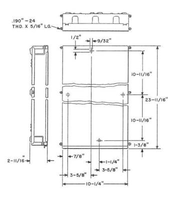
Consists of a light olive gray enamel finished sheet metal intermediate section having open ends provided with a removable cover. Knockouts are provided in the top and bottom of the box for bringing in cables or wires. Eight screws for mounting terminal blocks and six screws and nuts for fastening sections together are furnished.
