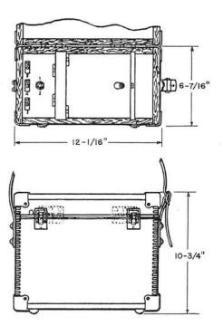
A portable test set consisting of a vibrator-type tone source, a motor driven interrupter, and associated apparatus mounted in a wood case. Continuous or intermittent tone can be selected by means of a switch. The set is powered by four ASA number 6 dry cell batteries which are not furnished.
