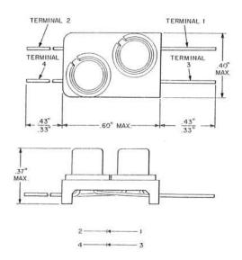
Each consists of a pair of silicon diffused-junction planar diodes matched for forward impedance and enclosed in a two-lead encapsulation.
