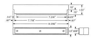
A wooden mounting strip equipped with a black finished metal retaining strip. Arranged to mount a strip of printed figures under the face strip.
