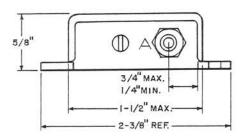
Designed to operate on either ac or dc voltages. Each buzzer has one coil, an exterior screw for adjusting the contact gap, and two exterior binding posts. The base and press on cover are of magnetic material.
