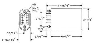
Shell type coils enclosed in metal cases. Operate over voice frequency range. Closest recommended mounting centers are 3-3/16 inches by 1-3/4 inches.
