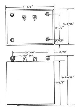
Consists of windings on a silicon steel core potted in a metal case. The closest recommended mounting centers are 3-11/16 inches by 4-7/8 inches.
