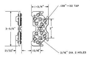
A block of insulating material equipped with ten screw terminals and arranged for number 101 type covers.
