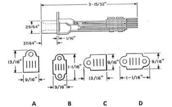
Single mounted, electrically welded frame type jacks are to be mounted with springs in vertical plane as indicated in Figs. A, B, C, and D. The letters A, B, C, and D used in code numbers of the jacks indicate number of mounting lugs and their arrangement with respect to the plane of the springs. Figs. A, B, C, and D illustrate the four arrangements of lugs and springs as indicated in code numbers by the letters A, B, C, and D, respectively.
