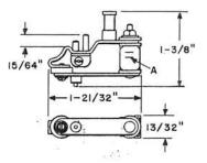
Intended for use with the W4AG and W4P Cords as test plugs in connection with the protectors of main distributing frames of manual and dial offices.
