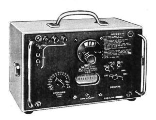
A portable transistorized battery operated test set enclosed in a metal case. The dimensions are 9-1/2 inches high by 13-3/4 inches long by 10 inches wide. Weight is 15 pounds (including batteries).
