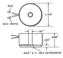
Consists of a winding on a permalloy powder core and potted in a case of insulating material. Provided with flexible terminal leads approximately 8 inches long. Inductance values are from 0.00200 henry to 2.23 henrys. The nominal inductance desired must be specified in the order to not more than three nor less than two significant figures.
