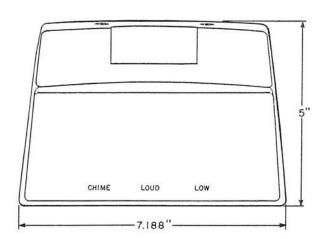
Plastic ivory covers each arranged to mount on an F1A Ringer. Bottom surface is slotted to permit sufficient gong sound output and recessed to permit access to the signal lever. Captive mounting screws are furnished.
