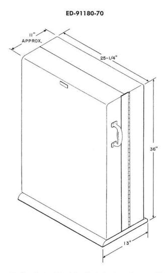
Metal cabinet with a hinged steel gate and removable metal cover. The cabinet is arranged for wall or floor mounting. Has a capacity of 18 mounting plates 14-1/8, 19, or 23 inches long by 1-3/4 inches wide. Consists of cabinet groups 23, 24, 28, 30, and 32; wooden base groups 18, 29, and 31; nameplate group NP; and mounting framework groups 3, 4, 5, 6, 9, 15, and 16. The groups required as described below must be specified on the order.
