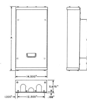
Each consists of a sheet metal intermediate section provided with a door. The door is provided with slot type knockouts for cable entrance. A wooden backboard, equipped with wiring brackets and distributing rings, is mounted in each cabinet.
