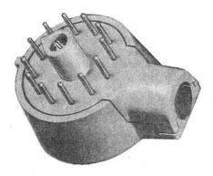
Consists of a block of insulating material containing 12 terminals and a removable cap. Each terminal is equipped with a spring connector which permits friction contact with number 134 or equivalent cord tips. Has a slotted guide for guiding the cord tips into the spring connectors.
