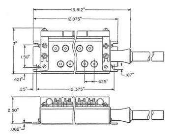
Consists of an olive green enamel finished sheet metal sealing chamber having an insulating panel equipped with 16 pairs of binding posts with associated nuts and washers. Furnished with a 12-foot number 19 AWG quadded stub cable.
