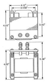
Consists of a winding on a grain oriented silicon steel core clamped between metal brackets which provides a means for mounting.
