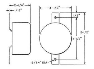
Cylindrical plastic case with black semiflexible insulated snap-on cover for potting one 652, 658, 659, 641, 642, 643, or 644 Loading Coil or a 1574A or B Inductor. Equipped with four 2A1B Protector Units for protection against lightning or heavy surge currents. Mounting screws are provided for pole mounting.
