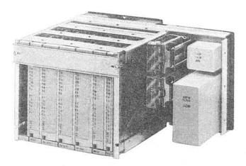
A low-speed, non-integrated data set capable of fullduplex operation over a four-wire voice frequency circuit. It is designed for the transmission and reception of signals of a multifrequency 2-out-of-10 code format.
