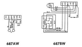
687AW-49: A common battery set having a terminal block and a metal base on which is mounted a C4A Ringer and a 548A Capacitor. The set has a light olive gray plastic cover assembled to the base.
