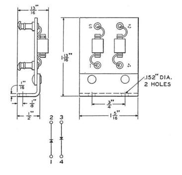
Multiple semiconductor type, consists of two selected number 400 type diodes mounted on a plate of insulating material assembled on a metal mounting bracket.
