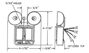
Unit type biased ringer having a cantilever type biasing spring arranged for three settings and a stroke adjusting stop for adjusting the sound output. The dc resistance between slate and black leads is 960 ohms  $\pm 10$  percent, between red and slate-red leads is 3640 ohms  $\pm 10$  percent, and between red and black leads with slate and slate-red
