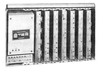
The Data Set 105CW1 is a frequency shift receiver and transmitter designed to convey teletypewriter information. Two frequency shift channels are used. The set operates at 100 words per minute. Intended for 8 level M35 Teletypewriter automatic send and receive operation. The set provides for alternate voice communication.
