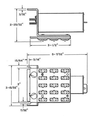
Arranged to mount in a number 105BW Apparatus Box. Requires angle type P-37B204 Bracket for installation on 16C Apparatus Mounting or when unit is relay rack mounted.
