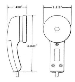
Consists of a moss green thermoplastic receiver handle and cap equipped with an HC3 Receiver Unit and R2FL-51 Cord.
