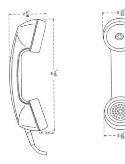
The G3-type hand sets consist of a P-80J200 Handle, a P-80A200 Receiver Cap, a P-80A100 Transmitter Cap, a TI Transmitter Unit and the apparatus shown in the table. CORD
