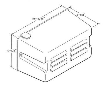
A molded fiber glass cabinet with a stippled light olive gray finish. Cabinet is wall mounted on a wooden backboard and has ventilation louvers and cable entrances. Used to enclose the 101J Power Plant.
