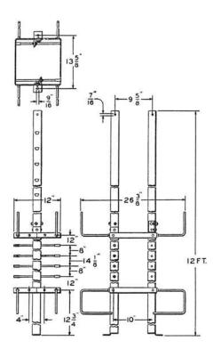
Consists of a metal framework for supporting binding post chambers and backboards. Provided with distributing rings and rods for supporting wires and facilities for attaching standard cable hooks. Sleeves, bolts, and nuts for fastening sections together and screws for mounting binding post chambers are furnished.
