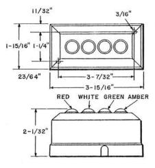
Four lamp indicator equipped with colored lamp caps. Housing is of insulating material and has a light olive gray finish.
