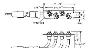
Gas tight cable terminal consisting of a metal plate equipped on one side with four KS-14743 Connectors and on the other side with a tube assembly which is terminated with a four-pair video type lead covered polyethylene insulated stub cable having number 16 AWG conductors. Each
