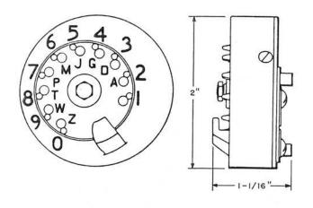
Provided with a finger wheel which when rotated causes a pair of contacts to make and break, thus permitting impluses to be sent into the dial system offices.
