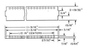
Hard rubber mounting that will accommodate 20 jacks. Furnished only on orders for jacks and unnumbered unless otherwise specified. Not furnished partially equipped with jacks. The lower edge of face is grooved and spotted.
