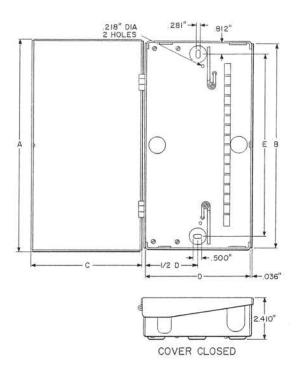
A sheet metal box with a hinged cover, having a light olive gray enamel finish. Provided with knockouts in both ends for cable and wire entrance. Also provided with a fanning strip and two 8A Distributing Rings. Screws are provided for mounting a terminal block or an adapter.
