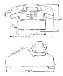
A black common battery desk type TOUCH-TONE telephone set. Equipped with a jack to provide for head telephone set or hand set operation. Equipped with a 253A TOUCH-TONE Dial, a G3AR-3 Hand Set, an N1A Ringer, a 642A Key, a D10P-3 Cord, a 241A Amplifier, a 425G Network, and a 100A Varistor. If Head Telephone Set is required, it must be ordered separately. A snap-on plastic face plate, arranged to accommodate a number card, is mounted on the top side of the housing.
