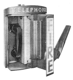
The telephone is enclosed in a red weatherproof aluminum housing, 16-7/8 inches high by 12 inches wide by 7 inches deep. Front is made up of double doors hinged at the center. One door provides access to the telephone. The other door is screwed shut and provides access for maintenance.
