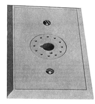
Consists of a 541A Jack, a 43B Bracket, and a flush type cover plate arranged for mounting in a standard electrical outlet box. The associated 504A Plug can be inserted in one position only. Overall dimensions of the 547B are 4.500 inches long by 2.750 inches wide by 1.384 inches deep.
