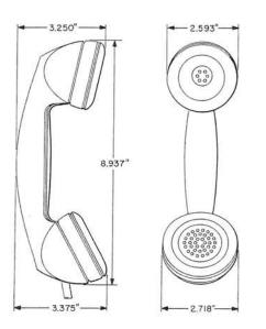
Black finished hand sets consisting of an F1 Transmitter Unit and a LA3 Receiver Unit.
