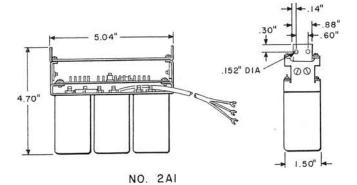
These are reverse channel units used as circuit assurance, line break, or low speed serial reverse information channels.
