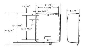
687CW-49: Similar to 687AW-49 except a 198C Capacitor is mounted on the metal base plate and the ringer is not furnished. The approximate overall dimensions are 5-1/2 inches wide by 6-13/16 inches high by 2-3/4 inches deep.
