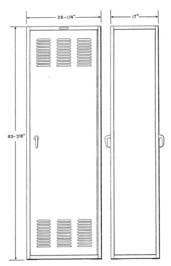
A floor supported common systems steel cabinet with doors opening to the front and rear. Consists of cabinet groups 6, 15, 16, 17, and 18 and nameplate group NP. The groups required as described below must be specified on the order.
