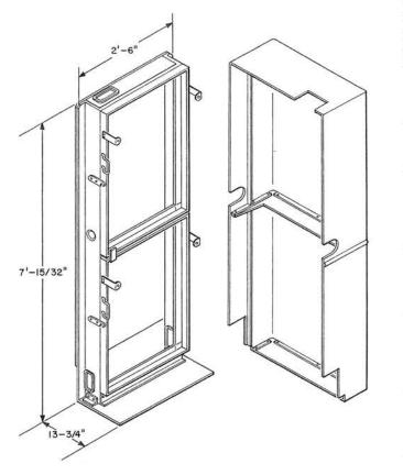
A station systems wall relay rack with two gates for ready access to mounted apparatus arranged for mounting forty 1-3/4 inch mounting plates 19 or 23 inches long or thirty-four 2 inch mounting plates 23 inches long. Optional mounting materials consist of Groups 2, 3, 4, and 5. The groups required as described below must be specified on the order.
