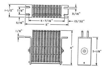
Silicon carbide disc type varistor with ten groups of discs, each group having two discs and three terminals. The center terminals of the ten groups are strapped together. Screws for mounting are furnished.
