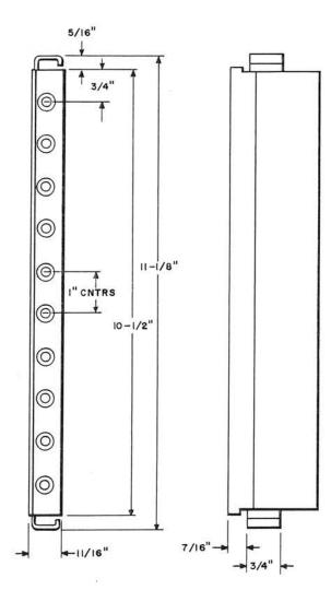
Metal mounting with a face of insulating material that will accommodate 10 jacks. Furnished only on orders for jacks and unnumbered unless otherwise specified. Not furnished partially equipped with jacks. The lower edge is grooved.
