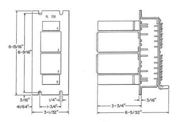
Terminal panel has 40 terminals, arranged in 4 rows of 10 each, numbered 1 to 40.
