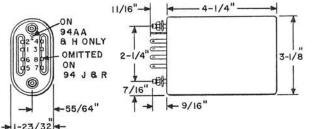
Consists of shell type coils enclosed in metal cases. Arranged to mount on mounting plates. Closest recommended mounting centers are 3-3/16 inches by 1-3/4inches. Potted, unless otherwise specified.
