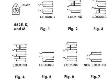
Nonlocking push button keys in a case of insulating material. Push button is white plastic. Provided with window having a transparent face strip for mounting a designation card.
