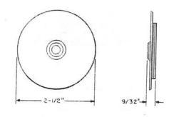
An adapter of black insulating material for use in replacing the receiver caps of operators' head sets to provide for a 101A Pad.
