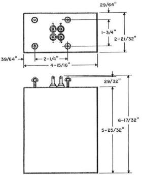
Unbalanced band-pass filters consisting of inductors and capacitors enclosed in a metal can. Arranged to pass a band of frequencies about 110 Hz wide with its midfrequency located as shown in table.
