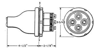
Gas tight cable terminal consisting of a cylindrical coupling provided with a four shielded pair number 19 AWG stub cable 15 feet long. Each pair of conductors is connected to a soldering terminal provided with a shielding cap.
