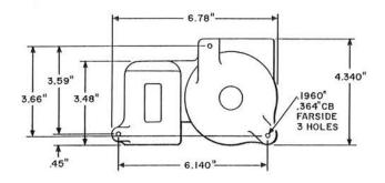
Consists of a subharmonic generating transformer, capacitor, diode, and resistor. The parts are enclosed in an epoxy filled plastic case. Input and output leads extend from solder type terminals recessed in the case. It is arranged to be an integral part of the 20AW1 Power Unit which may be mounted within a cover on system framework or wall mounted within a ventilated cabinet. It weighs approximately 3 pounds.
