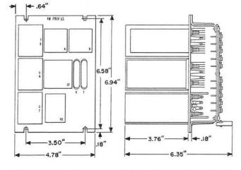
Terminal panel consists of two groups of terminals. One group has 40 terminals arranged in 4 rows of 10 terminals each, numbered 1 to 40. A second group has 20 terminals arranged in 2 rows of 10 terminals each, numbered 1 to 20.
