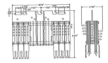
This jack is used in central offices located in areas where incoming circuits are underground and do not require heat coil and block protection. Cable capacity is 100 pair. Jack provides a ready means of opening lines and trunks for test purposes.
