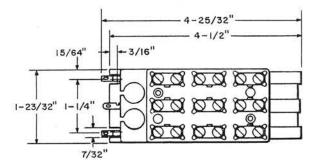
These are resistor units for dc lamp supply.
