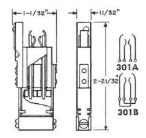
301A: A test plug with contacts insulated from each other. Provided with sleeve and spring for holding the plug in position in jack. Can be used on right or left side of jack. Engages with number 444 or 452 type jack. Used with P2BK and W4AL Cords.
