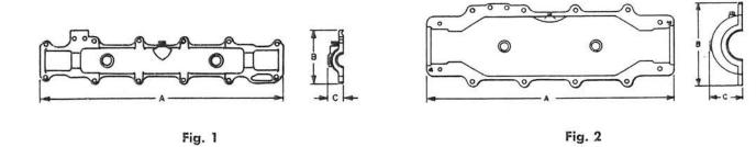
Each consists of a cast metal housing with a semicylindrical cavity. Provided with a pipe plug for pressure testing. Used as part of a gas and moisture tight splice closure for multiple sheath cable and lead covered cable of diameter indicated in table.
