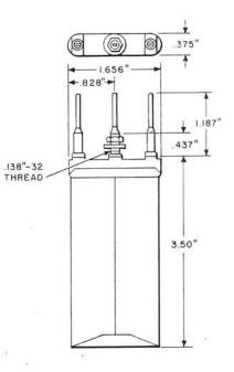
Two winding resistor. Each winding is wound on a nonmagnetic metal core. Has three terminals, the center terminal being common to both windings. Has a cover of insulating material. Terminals are tinned and are arranged for mechanically wrapped connections.
