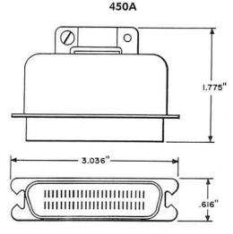
Consists of a rectangular block of insulating material equipped with 50 gold plated contacts assembled in a front and back metal shell which is equipped with a cable clamp located on the rear of the shell. Polarized to ensure proper mating with locking connectors. Intended for a maximum of 200 operations in a temperature range of  $+60^\circ$  to 120°F. (Nonoperating temperature range of -40° to +160°F.) Maximum operating voltages are 125 volts ac and 56 volts dc.
