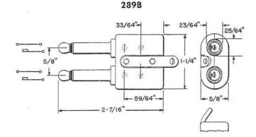
Flexible, twin double conductor plugs with black shells. Constructed so that there is sufficient play between the plug bodies to take up any variation between the jack centers and arranged so that each plug body may be turned 90 degrees in the shell to present a new surface for wear. Equipped with a bracket for cord stay.
