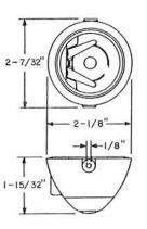
Black plastic case arranged to accommodate an HC3 or HC4 Receiver Unit. Provisions are made for attaching a transmitter arm and a headband to the receiver holder. Necessary receiver cap is furnished with the number 52 type head telephone sets of which this receiver holder forms a part.
