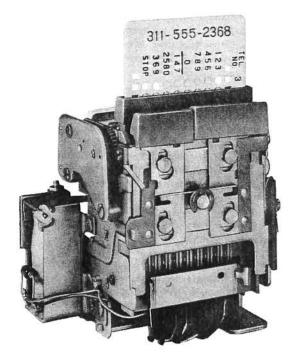
An electromechanical device which, when incorporated into a 660AW or 662AW type telephone set, permits an automatic dialing function. The telephone numbers of frequently called stations are stored in a repertory of punched cards (P-24E238), the blanks of which are furnished as part of the telephone set. Overall dimensions are 4.250 inches wide by 3.145 inches deep by 4.018 inches high.
