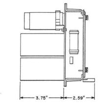
Terminal panel consists of a group of 40 terminals, arranged in 4 rows of 10 each, numbered 1 to 40.
