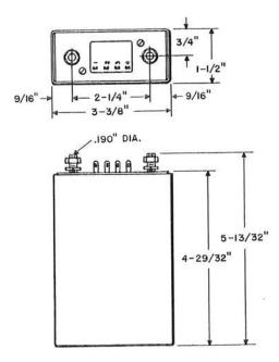
Balanced low-pass filters. Each filter consists of capacitors and inductors enclosed in metal can.
