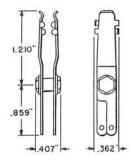
The 43A Lamp Sockets are strip-mounted and are furnished only on orders for lamp socket mountings.
