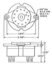
A flush-type jack consisting of a block of insulating material containing 12 contacts having clip-type terminals. Each clip terminal permits the connection of two insulated wires in multiple without removal of conductor insulation. Associated 504A type plug can be inserted in one position only.
