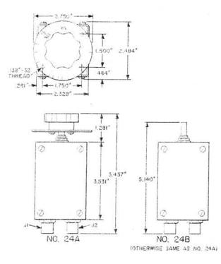
24A: Consists of a potentiometer, capacitors, and resistors assembled in a metal can. Two 509A Jacks are provided for external connections. The outer conductors of the jacks are grounded to the can.
