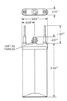
Single winding resistor. Winding is wound on a nonmagnetic metal core. Resistor has a cover of insulating material. Terminals are tinned and arranged for mechanically wrapped connections.
