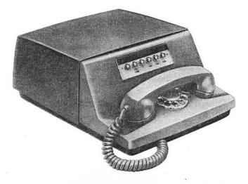
The Data Set 603BW3 is a narrow-band, low-speed, analog receiver used for reception of signals (0-100 Hz) from a 603AW1 or 603DW1 transmitter.
