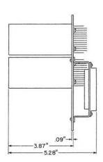
This unit is designed to mount on a 16C Apparatus Mounting. A KS-16672L1 Connector which has 50 contacts arranged in two rows of 25 provides plug-in connections when assembled in a key service unit.
