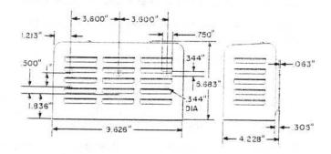
Consists of a metal bracket arranged to mount an L1AW-49 Ringer, and equipped with a removable louvered metal cover having a light olive gray finish. Provided with screws for mounting a ringer.
