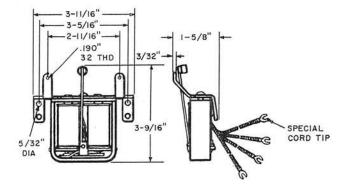
Unit type biased ringer having a cantilever type biasing spring arranged for three settings and a stroke adjusting stop for adjusting the sound output. The dc resistances between the red and yellow leads and the yellow and black leads are each 510 ohms  $\pm 10$  percent. All leads are 7-1/2 inches long.
