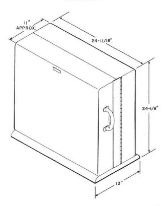
Metal cabinet with a hinged steel gate and removable metal cover. The cabinet is arranged for wall or floor stand mounting. The cabinet has a capacity of 11 mounting plates 14-1/8, 19, or 23 inches long by 1-3/4 or 2 inches wide. Requires one ED-91180-70, Group 29 light olive gray wooden base when floor mounted. Consists of cabinet groups 18 and 22; nameplate group 2; and mounting framework groups 3, 4, 5, 6, 7, 8, 13, and 14. The group required as described below must be specified on the order.
