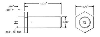
A single coaxial type, 75 ohm, hermetically sealed plug consisting of a metal cylindrical body having a metal contact finger assembled concentrically with the body by means of an insulator for connection to the associated jack at one end. The body, with the contact finger, is assembled to a gold plated metal shell which is positioned so that a portion of the body is exposed. The exposed portion is threaded for assembly to associated apparatus.
