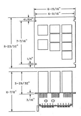
Terminal panel consists of three groups of terminals. Each group has 40 terminals, arranged in 4 rows of 10 each, numbered 1 to 40.
