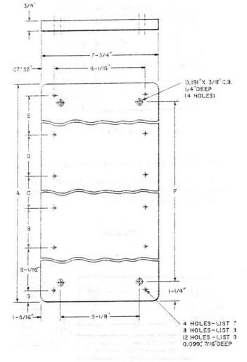
Particle board, light olive gray finish. List 7, 8, and 9 mounts 1, 2, and 3 number 105 type apparatus boxes, respectively.
