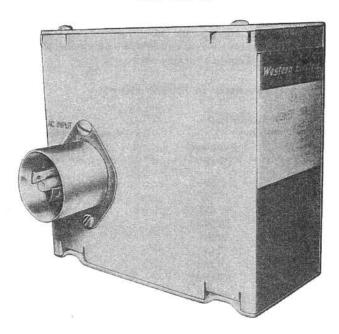
18A: Consists of a ferroresonant transformer, a diode, bridge, an ac capacitor, filter, capacitors, and resistors. The chassis and cover are aluminum.
