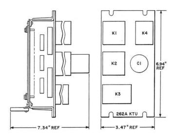
Apparatus assembled and wired on 228 Key Telephone Unit.
