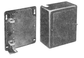
105BW: Metal box having an olive gray finish. Overall dimensions are 7.38 inches high by 6.88 inches wide by 3.38 inches deep. Two cable rings and two escutcheons are furnished. Intended to have key telephone units in the 1A1 Key Telephone System.
