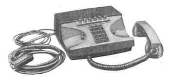
804GW1: Consists of a two-tone gray plastic housing containing an 11C Apparatus Unit, a 589T Key, three 52A Lamps, a D4BJ-61 Cord, an M14F Cord, and printed wiring boards containing component apparatus.
