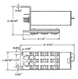
Arranged to mount in a number 105BW Apparatus Box. Requires angle type P-37B204 Bracket for installation on 16C Apparatus Mounting or when unit is relay rack mounted.
