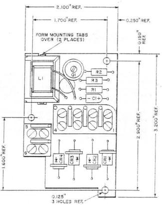
A single-stage transistor audio amplifier incorporating a polarity guard and consisting of apparatus such as capacitors, resistors, diodes, and an inductor mounted on a 0.062 inch thick printed wiring board.
