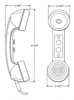
These plastic hand sets incorporate subminiature microswitches which serve to provide normal paths through the transmitter and receiver when operated, but short out the transmitter and receiver and shunt the cord leads through resistors when unoperated.
