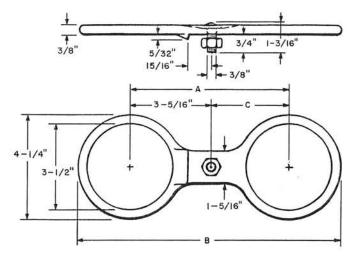
Vitreous enamel insulated metal rings used on distributing frames.
