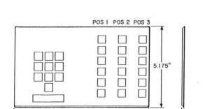
Clear plastic, nonglare type face plates each containing openings to accommodate a dial, key buttons and/or a transmitter, on associated telephone sets.
