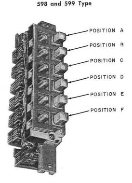
Mechanically locking keys consisting of plunger-operated spring combinations as indicated in table, and a common chaining switch, except where indicated by footnote, having three sets of break contacts wired to a KS-16672L3 Connector except where indicated by footnote. The buttons are of the illuminated type. Overall dimensions are approximately 6.594 inches long by 1.250 inches wide by 3.125 inches deep.
