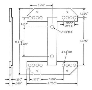
29C: A metal mounting intended for use in mounting telephone sets on buildings, fences, poles, etc.
