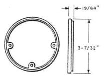
Consists of a spacer ring of black insulating material.
