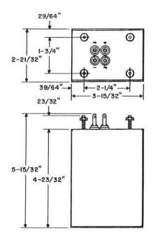
Unbalanced band-pass filters consisting of inductors and capacitors enclosed in a metal can. Arranged to pass a band of frequencies about 140 Hz wide with its midfrequency located as shown in table.
