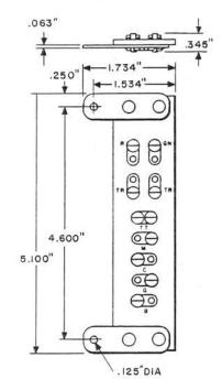
Consists of a strip of insulating material equipped with nine terminals and two mounting brackets. Used with 1A1 and 6A Key Telephone Systems.
