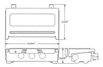
Consists of a cast metal housing having a hinged metal cover containing a connecting block equipped with six pairs of binding post and two terminals for ringing ground connections:
