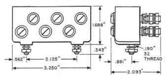
Each consists of a cast resin block containing three pairs of binding posts. Each binding post is equipped with insulation crushing washers to permit making cable terminations without removal of insulation.
