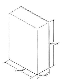
Designed for wall mounting a 26A Apparatus Mounting. Consists of a cover group 2, nameplate group NP, and a backboard group 3. The groups required as described below must be specified on the order. Assorted hardware used for mounting the 26A Apparatus Mounting is shipped unassembled.
