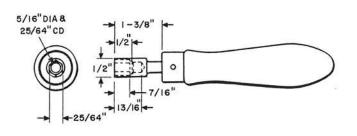
A socket wrench for use on hexagon cap nuts of relays. Comcode:  $100\ 750\ 405$
