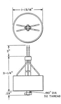
Plastic case arranged for potting one 642 Loading Coil or one 1574A or B Inductor. The code number of the loading coil or inductor required must be specified in the order. Case is equipped with number 19 AWG terminal leads.
