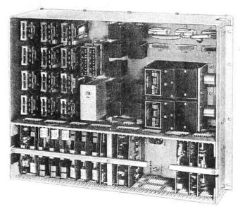
The Data Set 404AW1 is a low-speed parallel transmission transmitter and receiver unit.
