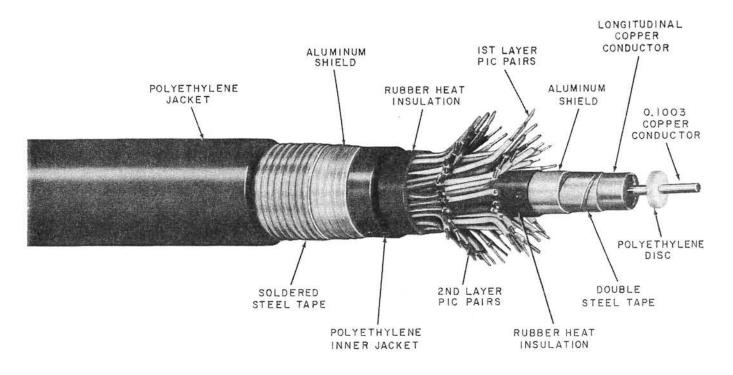
A cable consisting of one coaxial and a choice of 16, 37, or 63 PIC pairs of 19 gauge conductors. Intended for high frequency transmission.
