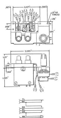
Consists of two push button operated spring combinations and a potentiometer assembled on a metal bracket. Equipped with a 51A Lamp for illuminating the plunger adjacent to the potentiometer. Terminals are approximately 18 inches long.
