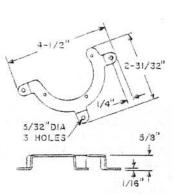
Semicircular flat metal plate with three mounting lugs. Screws, lock washers, and nuts are provided for mounting the dial adapter. Screws and lock washers are also provided for mounting the dial on the dial adapter.
