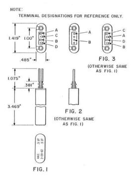
Metallized mylar capacitors potted in synthetic gel in aluminum cans. Minimum capacitance values are stamped on end of can unless otherwise noted.
