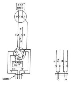
Black finished hand set consisting of F1 Transmitter Unit. LA3 Receiver Unit, H4BY-3 Cord, and 289B Plug. It is equipped with a push button switch in the handle. When the push button switch is depressed, the transmitter is connected into the circuit. May be obtained with a 13-foot cord when specified on order.
