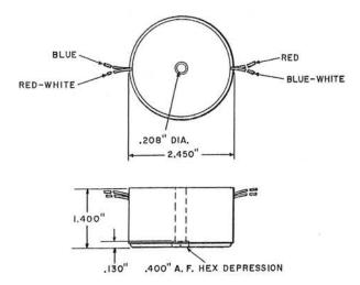
Consists of windings on a permalloy powder core and potted in a case of insulating material. Provided with flexible terminal leads approximately 8 inches long.
