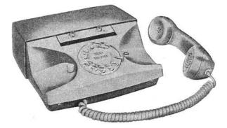
Each is an integrated set which combines a data transmitter, audible answer-back circuits, remote test circuits, and a telephone set in one housing. It is a low speed parallel transmitter in one direction delivering 3 to 14 frequency tones having a possibility of 99 different alphanumeric characters at a rate of 20 characters per second. Synchronization of timing is not required.
