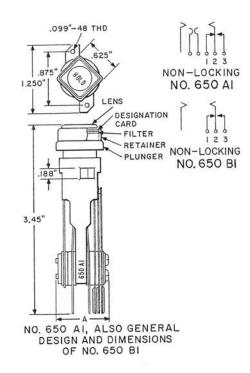
650A1: A nonlocking push button key. Equipped with a square-button plunger and retainer having a clear plastic lens. May be obtained with a green, red, or yellow lens when specified in the order. Contacts are of number 1 metal. Dimension A is 0.991 inch.
