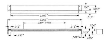
A wooden mounting strip with a black hard rubber face arranged to mount 20 number 17 Number Plates.
