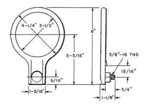
Vitreous enamel insulated metal ring used on distributing frames. Mounting screw and nut are furnished. Comcode: 100 666 635
