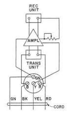
Consists of a T1 Transmitter Unit, an H4CT type cord with a vinyl jacket corresponding in color to the handle. Also contains a single-stage transistor amplifier, with a polarity guard, assembled on a printed circuit board which is fastened to a P14A464 Receiver Unit inside the handle.
