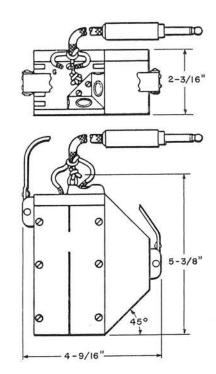
This unit consists of a single winding coil on a straight iron core enclosed in a wood case. It is equipped with a two bubble level, a W2CG Cord, and a 347B Plug for making external connections. It utilizes a tracing current supplied by a tone source such as a 20C or number 76 type test set.
