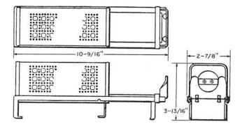
A rectangular cage; inner shield mounted on a base which may be used on a flat surface or fastened to a ladder step. Base extends beyond the cage and is formed to fit the handle of a soldering iron.
