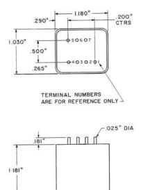
Consists of windings on a permalloy core, potted in a metal can and arranged to mount on printed wiring boards.
