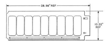
Consists of a fanning strip mounted on a terminal plate assembly 1 inch deep with a six foot AT-7441D Inside Wiring Cable.
