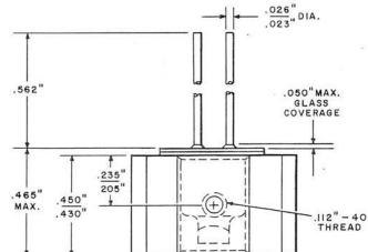
A P-N-P germanium alloy junction transistor assembled in a hermetically sealed metal can. A heat sink is attached to the transistor.
