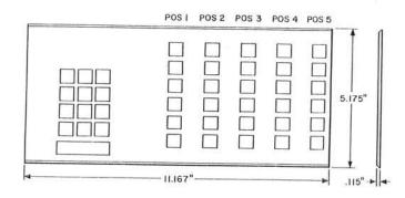
Clear plastic, nonglare type face plates, each containing openings to accommodate a dial and key buttons on associated telephone sets.
