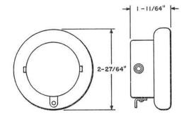
Watch case type receiver having a nickel plated metal case and a hard rubber cap. Resistance is approximately 1100 ohms.
