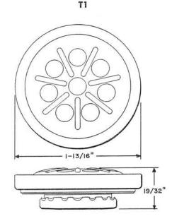
A carbon type transmitter unit intended primarily for common battery stations.
