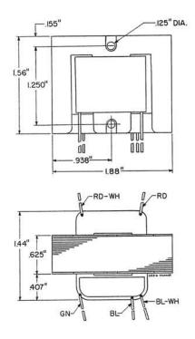
Consists of windings on a silicon steel core. Equipped with flexible terminal leads approximately 6 inches long.
