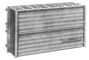
A four-wire, full-duplex modem that uses synchronous four-phase modulation for transmission of serial binary data at 600, 1200 and 2400 bauds per second. Transmission is over voice frequency circuits using a suppressed 1800 Hz carrier frequency. Available options include regeneration, choice of continuous or switched carrier, automatic answer, internal or external clock and power supply.
