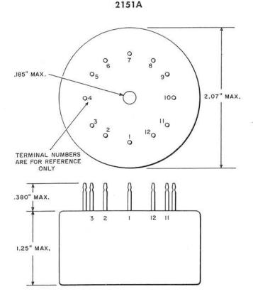
A toroidal transformer with a tape wound, oriented, 50 percent nickel-iron core cast in a cylindrical case of thermosetting resin.
