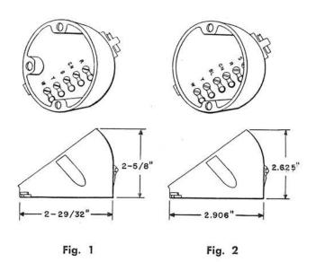
44B-3: Consists of black plastic frame provided with five contact springs, five screw terminals, and a 59B Dial Adapter. The springs are so positioned as to make contact with the contact points of number 25 type connecting blocks. A locking stud is provided for securing the dial mounting to the connecting block. Dials can be mounted at an angle of approximately 37 degrees from the horizontal. Arranged to mount 6E, 6F, or 6P type dials. Fig. 1 shows 44B.
