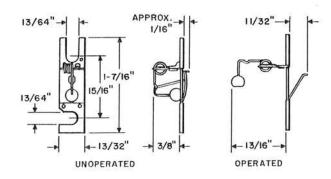
An indicator alarm type fuse mounting on 1-inch centers with tinned finish terminal. See table at end of fuse descriptions for capacities obtainable and operating current values.
