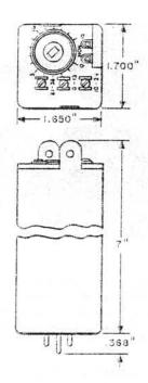
Each is a two-stage transistor, adjustable gain amplifler, consisting of apparatus such as capacitors, resistors, diodes, and transistors mounted on a printed wiring board and assembled in a metal can.
