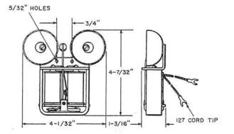
Biased type having a cantilever type biasing spring arranged for three settings and a stroke adjusting stop for adjusting the sound output. Equipped with 8-7/8 inch red lead and 6-7/8 inch black lead.
