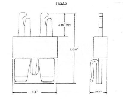
Consists of a block and a two terminal connector assembly which provides a mounting clip.
