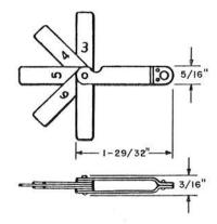
Consists of 75B through 75N Gauges mounted in holder. Individual gauges are readily removable and replaceable. Comcode: 100 863 760
