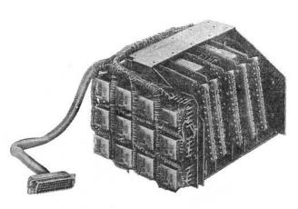
The Data Set 103EW5 is a full-duplex, phase modulated, serial data set which operates asynchronously at speeds up to 300 bauds. Meets EIA Standard RS-232A interface specification.
