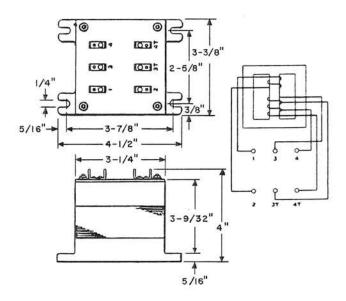
Shell type coils having a silicon steel core clamped between two cast iron end housings, one of which is provided with mounting lugs. Coils operate on a frequency range from 300 to 700 Hz.
