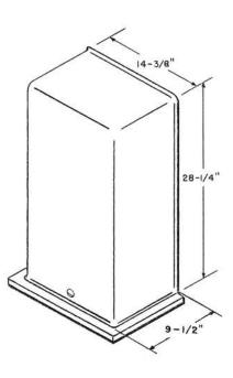
Designed for floor or wall mounted number 301 type key service units. Consists of a base plate assembly group 1, cover group 2, floor board assembly group 3, and nameplate group NP. The groups required as described below must be specified on the order. The floor board assembly is shipped separate; other assorted hardware remains unassembled until equipment is mounted.
