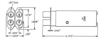
556A: Consists of two number 513-type twin coaxial jacks. One end is arranged for use with 358A or similar type plugs. The other end is arranged for use with 754E Cables. Each jack is equipped with a 62 ohm resistor and with a cable guard. Mounting screws are shipped loose.
