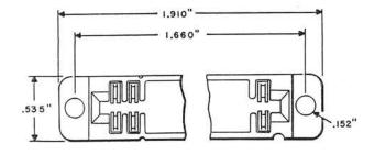
Consists of a molded block of insulating material containing 14 spring terminals in two rows of seven each. Equipped with twin contacts of No. 3 metal for connection to a printed wiring terminal.
