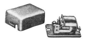
Equipped with heavy silver contacts and reed mounted armature with a flat retractible spring and stop. Overall dimensions are 1-1/8 inches high, 2-11/16 inches deep, and 1-31/32 inches wide. Light olive gray finish.
