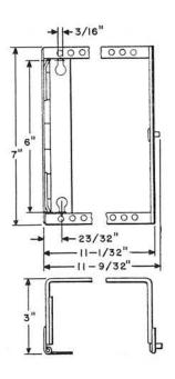
Metal framework arranged for mounting some 200 type key telephone units. Can also mount bent bracket type key telephone units by using P-37B204 Brackets. Brackets must be ordered separately.
