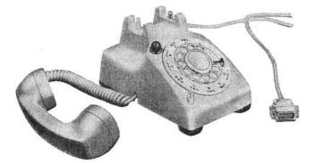
A common desk type telephone set which provides an interlock feature between the telephone line and a data set. The set is light gray and has overall dimensions of 8.297 inches wide by 9 inches deep by 4.906 inches high. The set has an exclusion type data key (left plunger) for voice-to-data transfer.
