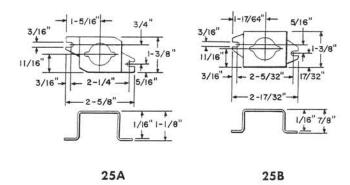
Metal brackets intended to mount stud mounted capacitors in place of lug mounted capacitors where mounting plates are drilled for capacitors having the mounting lugs located off center, 3/8-inch for 25A and 5/32-inch for 25B.
