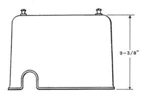
Light olive gray molded cover of insulating material having top and bottom cable openings. Arranged to cover one or two 15A Apparatus Mountings when mounted on a 173A Backboard. Provided with two cover supports and eight round head machine screws for assembly to the apparatus mountings, and with a dust guard and two round head wood screws for covering one cable opening.
