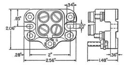
Consists of a base of molding material equipped with four 2B1A Protector Units.
