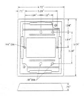
A molded gray plastic adapter, provided with mounting screws and two plates for reinforcing the mounting surface.
