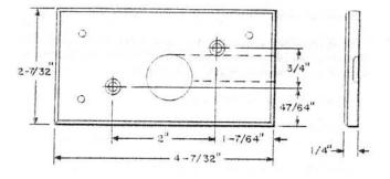
Phenol fiber backboard, light olive gray finish. Screws for mounting backboard to wall and indicator to backboard are furnished.
