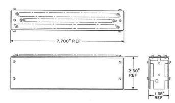
Consists of apparatus such as transistors, resistors, capacitors, inductors, transformers, and relays mounted on a flexible and rigid printed wiring board which is mounted on a frame with a common terminal strip forming a rectangular package.
