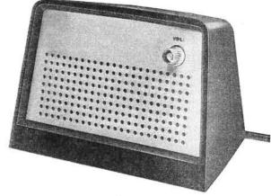
Consists of a KS-16881L5 Loudspeaker and a two-stage transistorized amplifier mounted on a metal base enclosed in a plastic housing. The knob controls an ON-OFF switch and a volume control potentiometer. Overall dimensions are 5.750 inches wide by 4 inches high by 3.750 inches deep.
