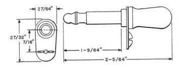
Solid metal finger plug with black insulated handle. Short circuits tip, ring, and sleeve of number 49 Jacks. Equipped with small shield which obscures light from lamp.
