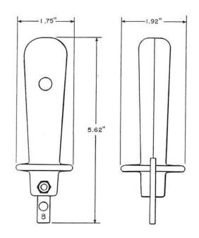
A hand tool having a plastic handle, containing a metal blade. The blunt end is for connecting a looped conductor, and the sharp end for terminating and cutting off a plastic insulated wire on a quick-connect terminal. One half of the handle is yellow to indicate the cutting side of the blade and the other half is green.
