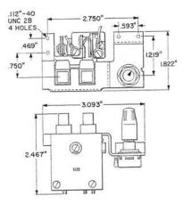
Consists of a two button ON-OFF Key with square buttons and a potentiometer assembled to a bracket for panel mounting. A clear plastic window and four .112-40 by 1/2 inch long FHM screws are shipped loose. The ON key is equipped with a 51A Lamp; and the key, potentiometer, and lamp are equipped with 18 inch spade-tipped leads.
