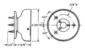
Consists of the 30A Dial Mounting provided with a black finished base for mounting dial in a vertical position on local test desk and PBX switchboards. Mounting screws are furnished.
