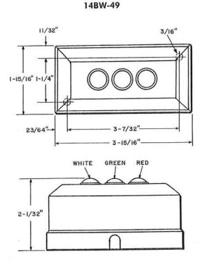
Three lamp indicator equipped with colored lamp caps. Housing is made of insulating material and has a light olive gray finish.
